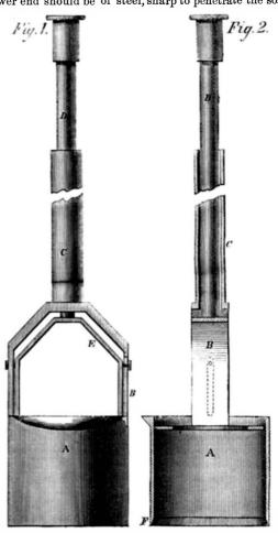
From two opposite sides of this cylinder, at the top, rise the arms, B, which are fastened to the hollow handle, C. Inside this hollow handle is a rod, D, terminating at the top in a knob, and at the bottom secured by the yoke, E, to a ring loosely fitting the interior of the cylinder. The upward and downward movement of this ring is guided and governed by pins sliding in vertical slots in the upright portion of the
