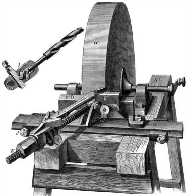
STRAHAN'S DRILL REST FOR GRINDING.
