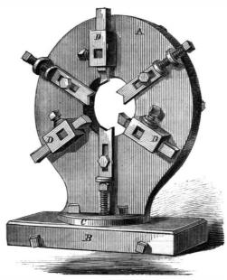
The object of the improvment is to avoid the trouble of removing bolts or studs from the lathe, after being turned, for the purpose of threading them in the screwing machine, which is a quicker way than that of chasing them on the lathe, but renders them liable to be threaded one sided.
