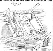
length of stroke imparted to them, and H is moved in the grooves by the rod, I, that is connected to the lever, J, which the workman operates by his foot and secures in the proper position by the rack, K, a spring pressing against I tending to keep it in the rack, and facilitating the back motion of G. The cutter will be better seen in the detached view, Fig 2, it is moved by the rods, O, on the toothed ways, a, that can be raised or lowered to regulate the thickness of the shavings, by
