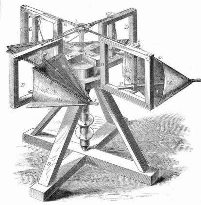
angles. The upper plates, a, when the wheel is not to be rotated are allowed to descend, the cords, l, being lowered, and the stops, o, will again pass over the upper plates, a, and prevent them from rising. In case the wind has great velocity, the wheel is prevented from having two great a speed in consequence of the valves, c, opening, the springs | him at Greenfield, Mass.
