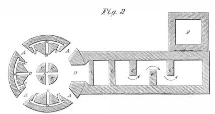
places, every portion of the fuel has a chance of being burned. The heated products of combustion pass through the flue, D, and over the bridge, b, giving up their heat to the boiler, and also in the direction of the arrows in Fig. 2, around the side bridges, e', so that no heat may be lost. There is a damper, f, at the side of the chimney, which directs the
