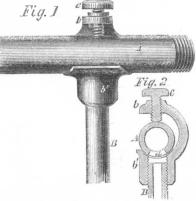
When gas or water pipes are laid, much time and labor are expended, and consequent expense incurred in joining the branch pipes to the main, and in connecting the supply pipes to the branch. The branch pipes are usually cut in two, their ends are then cut
