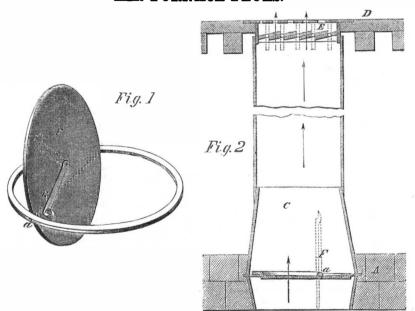
A great objection to the use and adoption of air-heating furnaces is that the hot air conducting pipes are very liable to become overheated when the registers are closed; and from this cause many serious accidents have going on. There are also openings for clean- coccurred, the adjacent wood-work taking fire, the pipes is closed, and the draught through this bridge.
