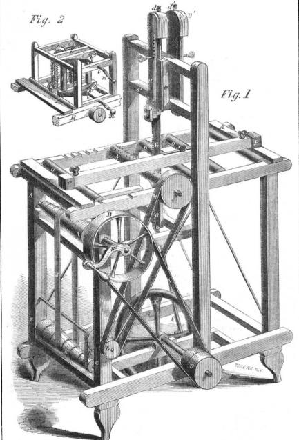
The inventor of this machine-D. B. Bar- | attached to the frame, A, and guides, b, attholomew, of Lancaster, Pa.—has produced a compact arrangement of parts that will enable any one to have a good sawing machine in their workshop, not only at a low price, but also one which requires but little power, as he makes them from small enough to be operated by hand, up to any size required.
