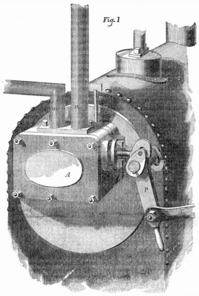
ratus for supplying steam boilers with water, water is supplied. r and r' are the valve for which a patent was granted to Benjamin stems respectively, which are actuated by F. Bee, on the first of August last, to which the rocking shaft, T, and lever, P, fig. 1. It is he has given the title of Hydrestant. Figs. 2 and 3 are sectional views of the apparatus, showing the internal arrangements and the different positions the two valves are made to occupy, by which contrivance water is
