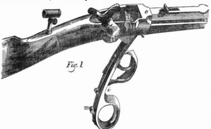
concentrate the fire upon the charge, in con- | er i, within a slot, i, in this lever. sequence of the nipple's being forced slightly within the surface of the end of the cart-
