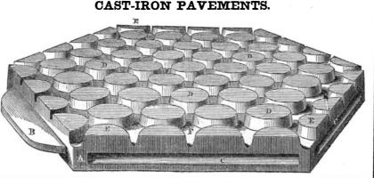
To supersede the ordinary Russ paving for, mortice or groove, C, let into it, into which iron blocks has been invented by L. Colwell, of New York City, who has taken measures to secure a patent. The above engraving is a perspective view of one of the blocks forming a section of the paving and displays the structure and arrangement of this new method Each of these blocks is six-sided, being in shape a regular hexagon, so that they are easily fitted one to another.
