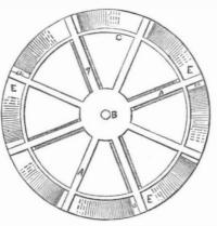
wheel has four sets of radial arms, A A A A. the shaft, B, and bound together by bolts to the rings, C C C C. The paddles or buckets, the form of the section of a flat ring, the cir- of the blades with the opening between them, expense of three hundred dollars.
