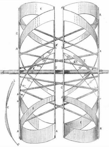
This paddle wheel for steamships and | cumference of which is equal in diameter to teamboats, is the invention of Abner Chapman, of Fairfax, Franklin Co., Vt. A patent was secured for it last year in England.
