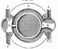
side of the engine, by a spindle passing through the top. D is a piece of chilled iron in the cock to resist the friction of the revolving cylinder, as explained in last figure. E is the steam passage and F the passage to the condenser.
