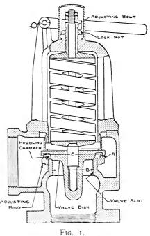
perhaps several fittings between it and the boiler. When the valve is closed the pressure in this pipe and directly beneath the valve will be the same as that in the boiler. When the valve opens, however, and a flow of steam occurs, the pressure at the safety valve end of the pipe will be less than at the boiler simply because there must be a difference in pressure to cause a flow of any vapor, gas or liquid from one point to
