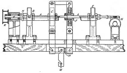
FIG. I. ROTATING BEAM TESTING MACHINE (FARMER).
