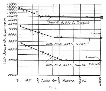
jecting the "normalized" steel to a heat treatment consisting of heating to  $1450^{\circ}$  F., holding 15 minutes, quenching in oil, reheating to  $1200^{\circ}$  F., holding 30 minutes and then cooling in air, a structure known as "sorbite" was developed in the steel. This "sorbitic" steel was found to have an endurance limit 84% greater than the "pearlitic." By still a third treatment which developed a structure
