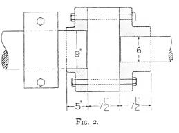
The face of this coupling was turned down so as to be at  $90^{\circ}$  with the shaft. The line shaft directly connected to the engine shaft was advanced so that the distance between the faces of the couplings was reduced to 4 inches for reasons which can readily be perceived.
