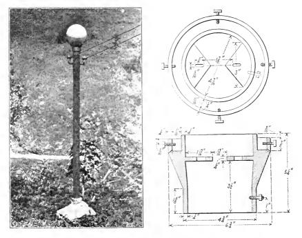
LIGHTING POST MADE FROM AN OLD BOILER TUBE, AND CASTING ADAPTING IT TO A STANDARD GLOBE.
