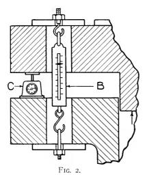
pull down on the cord until the scale reads 25 lbs. This represents the tension in the cord. Now place the 10 lb. weight on the scale pan. It will be seen that the tension in the cord is reduced to 15 lbs., but the scale reading remains unchanged.
