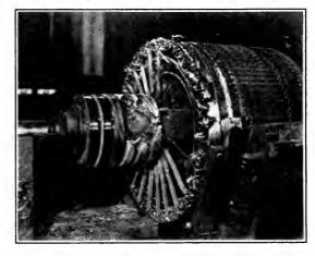
Armature Burnout of Rotary Convertor.
