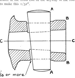
assembled, will not have a full bearing over its entire length and severe local stresses may be set up.
