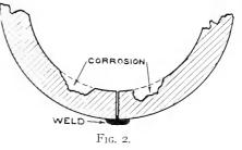
addition, as can be plainly seen in the picture and as indicated in Figure 2, serious corrosion had taken place forming deep grooves parallel
