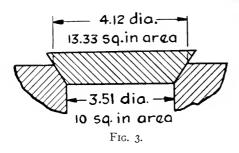
when it passed between the surfaces of the valve and the valve seat. However, some such increase in the total lifting force of the steam is effected and the excessive and uncontrollable amount of blowdown which results was one of the reasons for this type of valve being discarded.
