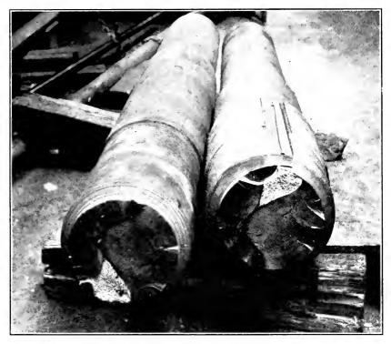
FAILURE OF SHAFT CAUSED BY WELDING.
