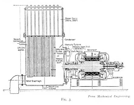
is no lower tube sheet. This construction takes care of the unusual expansion due to the higher temperatures, and gives a large heating surface with small volume of liquid.
