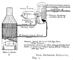
vapor is condensed in a surface condenser, the condensate then being returned to the boiler. just as would be done in any steam plant. It is interesting to note at this point that no feed pump is necessarv as the turbine is located above the boiler and the weight of the mercurv is such that it
