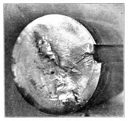
FRACTURE OF ENGINE SHAFT.
