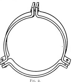
stack by means of an iron ring made as shown in Fig. 2 and at the lower end are secured to a building or to an anchor, such as a heavy block of concrete, buried in the ground. If but one set of guys is used, the ring in the stack is usually placed at about twothirds of the height above the base. If two sets are used it is common practice to place one at 2/5 and one at 4/5 of the height.
