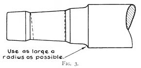
rubbed off and should be carefully filed down with a fine cut file until a neat fit is obtained over the entire length of the taper. It will be noted that no small degree of skill is
