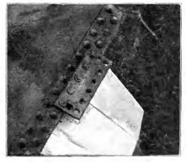
call a "Hartford" in- Soft Patch Used in an Unsuccessful Attempt to Repair a Longitudinal Seam Crack.
