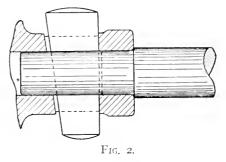
This space is for the "draw" and will be taken up when the key is driven in thereby providing a snug, tightly fitting joint. The amount allowed for this "draw" will vary with the size of the rod and the degree of taper. On large diameter rods not so much would be allowed as on small rods. With a rod diameter of  $2\frac{1}{2}$ " about 1/16" would be correct. If the rod has a cylindrical end, the two parts should go together with what a machinist terms a "push fit."
