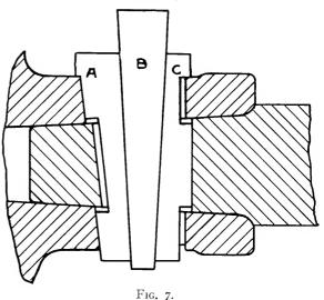
son the key should be a close fit on the sides but should have a clearance at the top. If this clearance is not provided, the load, when the hub bolts are tightened up, will be concentrated over the key, and the stresses tending to break the hub will be very much greater
