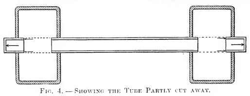
ment shown in Fig. 3, there *will* be a lengthwise stress on the tube, and its **amount will** be just equal to the pressure exerted by the water against the end of the tube.
