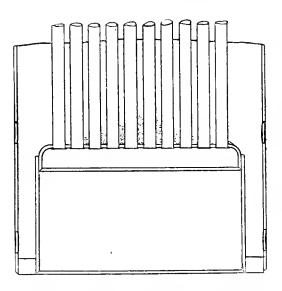
FIG. 2. — LOOSE DEPOSIT ON TUBE Sheet.
