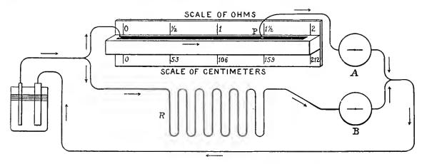
FIG. 7. --- Illustrating the Measurement of Resistance.
