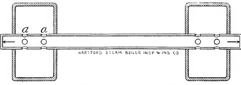
FIG. 3. - A PAIR OF DRUMS WITH PERFORATED TUBE.
