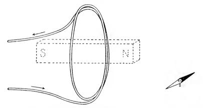
FIG. 1. -- ILLUSTRATING THE PRINCIPLE OF THE GALVANOMETER.
