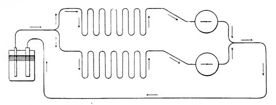
FIG. 6. - Illustrating the Principle of the Branched Circuit.
