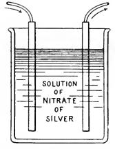
the rate of 0.071 ounces per hour, we say that it has a strength of half an ampere; and so on.
