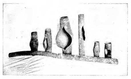
BURSTED BRASS BLOW-OFF PIPES.
