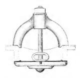
FIG. 5. — USUAL METHOD OF SECURING THE COVER PLATE.
