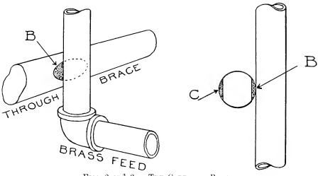
FIGS. 2 and 3. - THE CORRODED BRACE.
