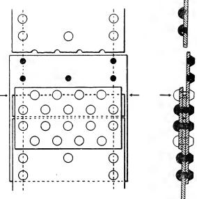
FIG. 4.—FRACTURE THROUGH THE NEXT-TO-INSIDE Row of Rivers.
