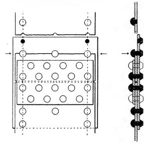
FIG. 3. — FRACTURE THROUGH THE NEXT-TO-OUTSIDE Row of Rivets.
