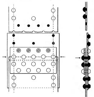
FIG. 5.— FRACTURE THROUGH THE INSIDE ROW OF RIVETS.
