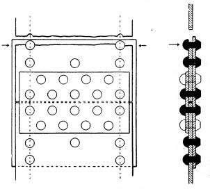
FIG. 2.— FRACTURE THROUGH OUTSIDE ROW OF RIVETS,
