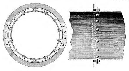
FIGS. 4 and 5.-RING OF ANGLE-IRON, WITH THIMBLES.
