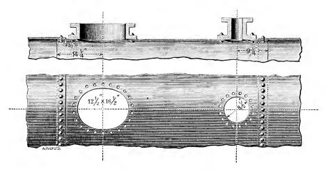
FIG. 1. - FAULTY LOCATION OF A MAN-HOLE.
