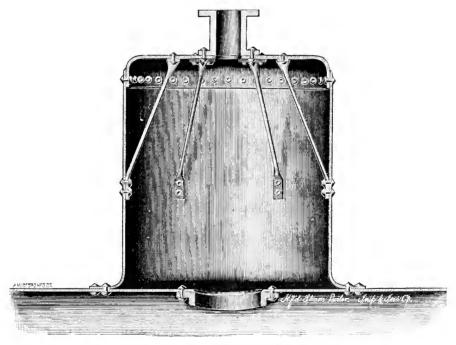
A CORRECTLY DESIGNED DOME.
