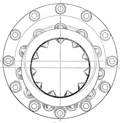
Fig. 22 shows in section a form of reducing coupling which could be used with advantage on all sizes of pipe up to eight or ten inches in diameter. Figs. 23 and 24, end and side views, of flange couplings for the larger sizes of pipe. The construction will be readily understood from an inspection of the cuts. The offset is just sufficient to bring the under sides of the pipes on the same level.
