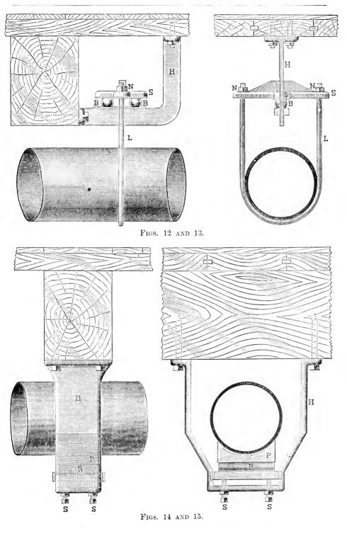
of the plank. The pipe is suspended from these bolts by means of bar, roll, and clips exactly as in Figs. 5 and 6, and the same facility of adjustment in a vertical direction is obtained as in that design.
