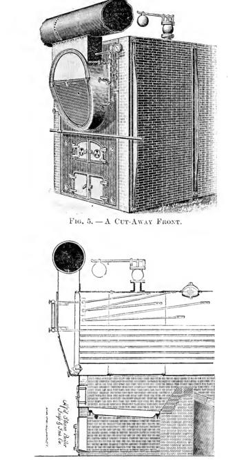
FIG. 6. - SECTIONAL VIEW OF A CUT-AWAY FRONT.
