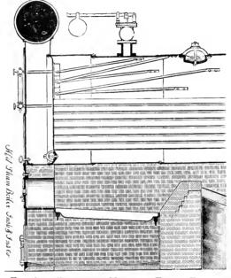
FIG. 2. - SECTIONAL VIEW OF FLUSH FRONT.
