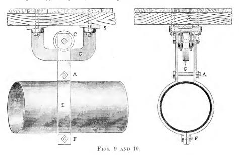
the timbers. In this case the weight of pipe would be carried by the floor planks instead of the beams. With mill floors as constructed at the present time, this would form a good support, especially if it were placed close beside a beam. Two bolts are
