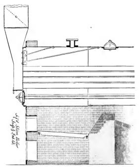
FIG. 2.— BOILER FRONT WITH BREECHING. SECTIONAL VIEW.
