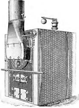
FIG. 1.- BOILER FRONT WITH BREECHING.
