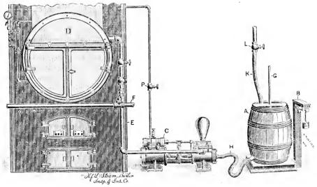
FIG. 1. - APPARATUS FOR EVAPORATIVE TEST.
