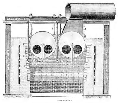
FIG. 1. - SETTING BOILERS OVER A SINGLE FURNACE.
