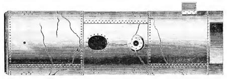
FIG. 4. - PLAN VIEW OF THE RESTORED BOILER.
