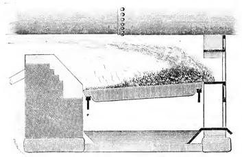
FIG. 3. BAD FIRING. - SIDE VIEW OF FURNACE.
