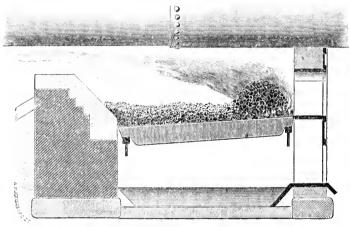
FIG. 2. COKE FIRING WITH SOFT COAL.
