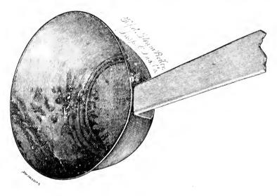
FIG. 1.-CORROSION FROM STANDING WATER.
