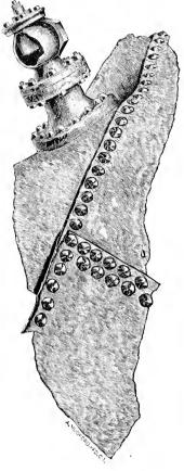
Many of the most destructive explosions of which FIG. 6. — THE SAFETY VALVE. we have any knowledge, have been caused by an inoperative safety valve, an accumulated pressure, and a full supply of water in the boiler;
