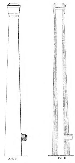
in Fig. 1, and the outer shell contracted to the area of the core, as shown in the engravings, but the better way is to run it up to about 8 or 12 inches of the top and *not* contract the outer shell. But under no circumstances should the core at its upper end be
