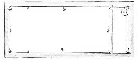
The accompanying cut shows the main features of the system, which, in this case, was put into a church, where, of all places, a perfect-working system seems to us desirable. The lower portion of the figure is a plan of the basement, the upper portion is a longitudinal section of the building, or rather of that part of it in which the heating arrangements were contained.
