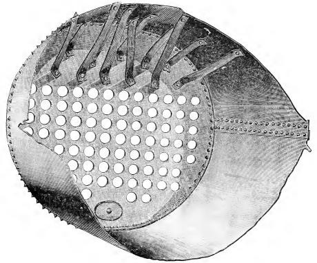
If we should construct an elastic model of an ordinary cylindrical boiler, apply pressure to it and carefully watch the effect, we should speedily observe the weakness of the heads by deflection or bulging. In some experiments made near Leeds, England, in 1876, described in "Nicholls' Practical Boiler-maker," upon an unstayed wronght-iron boiler head, 30 inches in diameter, and  $\frac{3}{8}$  of an inch thick, the deflection carefully measured and recorded was as follows:
