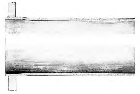
It should be stated that  $\frac{3}{8}$ -inch plate is thinner than is usually used for heads of boilers of ordinary dimensions. The thicker head or tube-sheet would give more frictional surface, and consequently more holding power. These specimens were handed to Mr. Charles B. Richards, Consulting engineer\* at Colt's Armory, in this city, with the request that he subject them to the required test.
