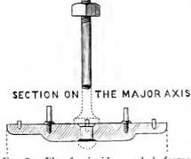
which is the first step in the process of fitting, the bolt - hole having been c o r e d with a square "counter - sink" to receive the head or clinch of the bolt as seen in section Fig. 7, and in plan Fig 8. The object of the square cavity ("counter-
