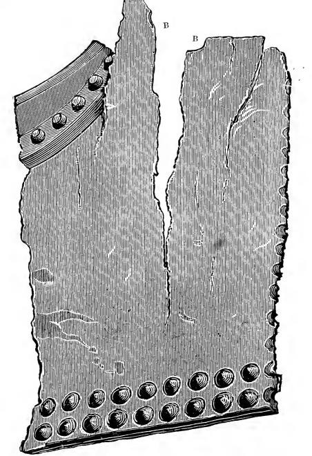
FIG. 6.—Part of the middle course of plates, boiler No. 3. showing broken manhole frame which struck and fractured boiler No. 2, splitting itself. Also showing at B B parts of the tapped hole through which the dregs pipe entered the boiler, as shown at B, Fig. 1.
