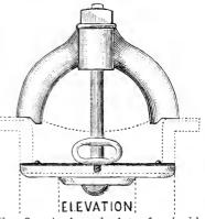
Fig. 7.— Plan for inside man-hole frame. sink") is to prevent the man-hole frame. rotation of the bolt in the plate when unscrewing the nut, which tendency will be realized if the threaded point above the nut becomes corroded so as to make the nut run
