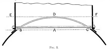
dome is of considerable size compared to the main cylinder, say 30" diameter on a cylinder 48" diameter, as here drawn, then a stay-bolt should be put across from B to C, fig. 2, which will effectually prevent motion and consequent leakage, as well as greatly strengthen the boiler shell on its weakest line.
