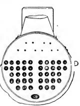
report, *i. c.*, putting in new second fire-sheet in second course. They have been in the habit of blowing off boiler, as soon as they hauled the fire; thus leaving boiler, while empty, exposed to intense heat of brick-work." We have repeatedly cautioned them against this and they now see the importance of it.
