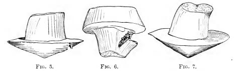
FIGS. 5, 6, 7.—Samples selected from a number taken from a "sheared" seam, which was believed to be the initial break from which the explosion arose. They were no doubt similar to Fig. 4 before they gave way. From photographs, full size.
