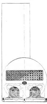
FIG.2.-Front elevation of the boiler, showing the opening in the tube plate made by the boiler-maker, shortly after the accident, for the purpose of remov-
