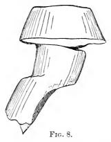
FIG. 8.—Rivet "driven" in over-set holes. Was probably fractured under the head in driving. Similar to Fig. 1. Taken from a seam that was broken through the rivet holes. From photograph, full size.
