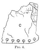
been subjected to violence greater than its fractious character would warrant, either at the time of being put upon the boiler or by the subsequent effort of the internal pressure to restore the distorted cylinder to a true form.
