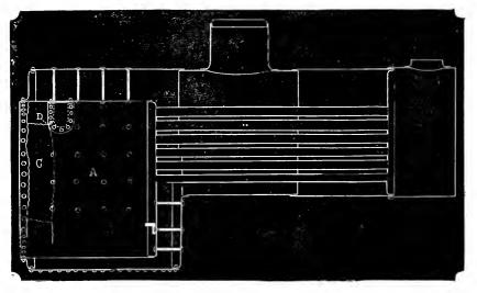
$F_{1G}$ , 2.—Longitudinal section of the boiler, showing lines of fracture of the left-hand wall of the fre-box, the corresponding end of the thin patch, and D, the probable point of initial rupture, indicated by the thin, pointed edges of the hole through which the head of the bolt was drawn, not shown in the cuts.
