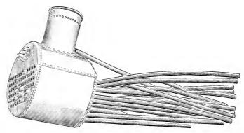
FIG. 3.-The rear end and tubes.
