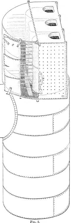
door, eighteen inches in diameter, opens into the port side of uptake.
