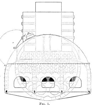
20 square feet, through which the entire contents of the shell issued at a temperature and velocity due to about 40 pounds per square inch of steam pressure, carrying away about 20 feet in length of the three decks of the vessel and everything thereon.
