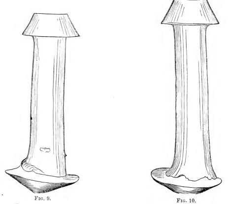
FIGS. 9 and 10.—Long rivets taken from a broken casting which they were intended to secure to the wrought-iron head of the boiler. The holes in the wrought-iron plate were "drifted" and chipped to allow the rivets to enter, as shown by the enlarged portion of the body. This irregular upsetting and the sharp little wave of iron on the body of Fig. 9 indicate the thickness of the wrought-iron plate. From photographs, full size.
