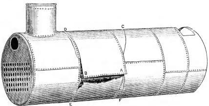
Fig. 1.—BA, line of initial fracture; AC, AF, BE, and BD, lines of secondary fracture, being the boundary lines of the detached ring of plates.
