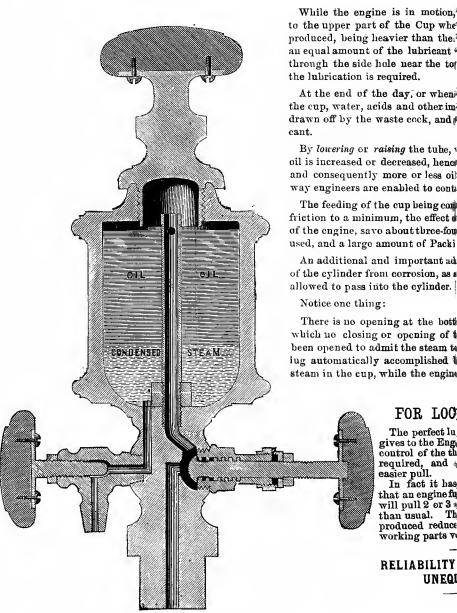
to the upper part of the Cup whe produced, being heavier than the an equal amount of the lubricant through the side hale near the tor the lubrication is required.
