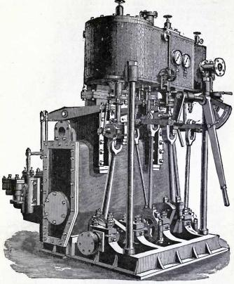
Fig. 368 .- Compound surface-condensing marine-engines, by Ross and Duncan, Glasgow.
