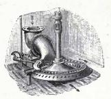
Fig. 13.—Girard-turbine with vertical shaft for high falls.
