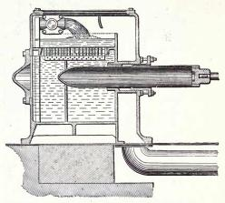
Fig. 184 .- Horizontal plunger-air-pump for a stationary engine.
