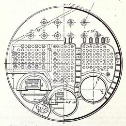
Fig. 125 .- Half-end view and cross section of the single-ended marine boiler, shown in Fig. 124.
