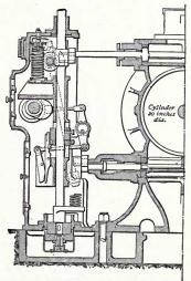
Fig. 237.—Corliss valve-gear by Hick, Hargreaves & Co., Bolton.
