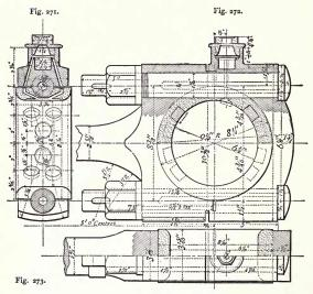
Figs. 271-273 .- Large end of the connecting-rod of a locomotive-engine.
