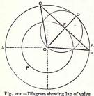
Fig. 212 -Diagram showing lap of valve and position of eccentric.
