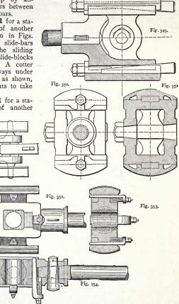
Figs. 348-354.-Crossheads of stationary-engines.
