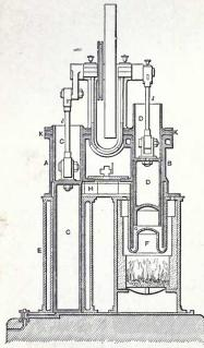
Fig. 19. - Rider's hot-air engine.
