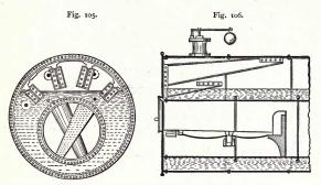
Figs. 105 and 106 .- Sections of a Cornish boiler, with Galloway-tubes.
