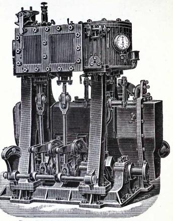
Fig. 261.-Yacht-engines with Bremme's valve-gear, by Ross and Duncan, Glasgow.
