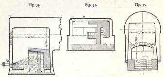
Figs. 33-35 .- Combustion-chamber for liquid-fuel.
