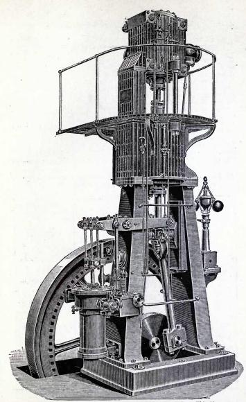
Fig. 365 .-- Vertical tandem compound mill-engine, by Douglas and Grant, Kirkcaldy.
