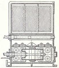
Fig. 185.-Horizontal plunger-air-pump with surface-condenser for a marine engine.
