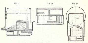
Figs. 36-38 .- Combustion-chamber for liquid-fuel.
