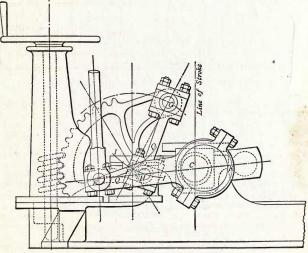
Fig. 260.-Bremme's valve-gear.
