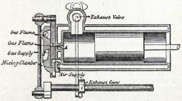
Fig. 18 .- Section of a cylinder of an "Otto" gas-engine.
