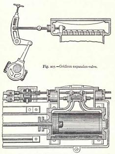
Fig. 208 .- Cylinder with separate expansion-valve.
