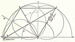
Fig. 214 .- Diagram of an expansion slide-valve.
