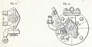
Figs. 22 and 23.-Urquhart's liquid-fuel injector.
