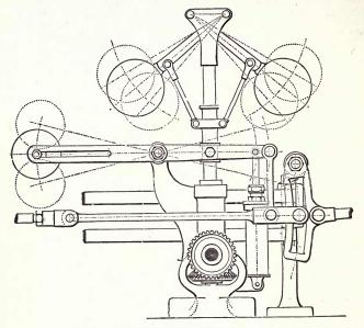
Fig. 367 .- Automatic expansion-gear of the engine shown in Fig. 366.
