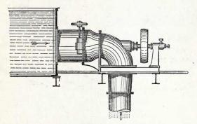
Fig. 9.-Jonval turbine, with horizontal shaft.
