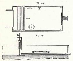
Figs. 190-192 .- Apparatus for measuring waste-water from condensing-engines.
