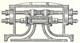
Fig. 213 .- Expansion slide-valve, with variable cut-off.
