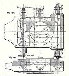
Figs. 278 and 279 .- Large end of the connecting-rod shown in Figs. 276 and 277.
