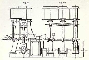
Figs 257 and 258 - Triple-expansion engines with Joy's valve-gear.
