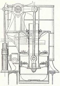
Fig. 186.-Trunk air-pump for a marine engine.
