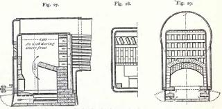
Figs. 27-29.-Combustion-chamber used in winter for liquid-fuel.
