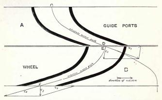
Fig. 6.-Diagram showing ports and buckets of a Jonval turbine, with water paths and velocities.
