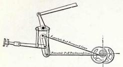
Fig. 243 .-- Link-motion with straight link.
