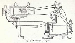
The engine works satisfactorily with common mineral oil. The quantity of oil consumed is about one pint per brake-horse-power per hour. When
