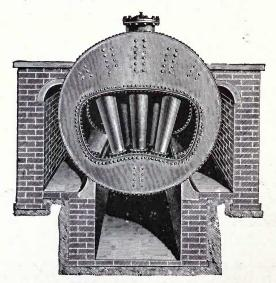
Fig. 116 .- Method of setting Galloway boilers.
