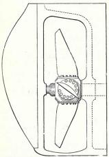
Fig. 307.-Screw-propeller with blades bolted to the Boss.
