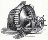
Fig. 14.—Girard-turbine with horizontal shaft for high falls. Cover removed.
