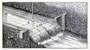
Fig. 3.-Notched-board for measuring flowing water.
