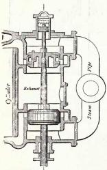
Fig. 229 .- Piston-valve of a marine-engine,
