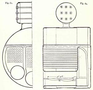
Figs. 61 and 62 .- Return tube marine boiler.
