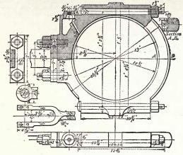
Fig. 248.-Eccentric-strap of a locomotive-engine.
