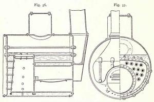
Figs. 56 and 57.-Return-tube marine boiler.
