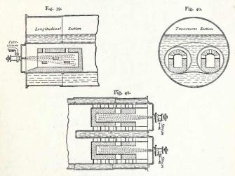
Figs. 39-41.-Combustion-chamber for burning liquid-fuel in Cornish-boilers.
