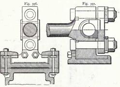
Figs. 356,-357.-Crosshead of a marine-engine.
