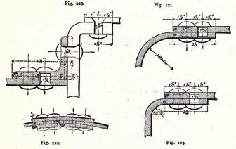
Figs. 120-123 .- Sections showing the riveted-joints of the locomotive boiler shown in Fig. 119.
