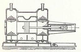
Fig. 183 .- Double-acting horizontal air-pump.
