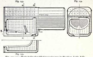
Figs. 133-135.—Marine boiler of modified locomotive type, by Hawthorn, Leslie, & Co., Newcastle-on-Tyne.
