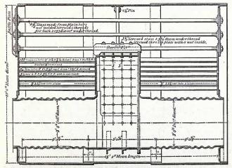
Fig. 127.-Longitudinal section of a double-ended marine boiler, by the Barrow Shipbuilding Co.
