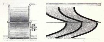
Figs. 7 and 8 .- Sections of the ports and buckets of the Jonval turbine.
