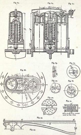
Figs. 83-94.-Details of safety-valve with Ramsbottom's lever and spring.
