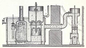
Fig. 172 .- Vertical jet-condenser, with air-pump and cold-water pump, for a beam-engine.
