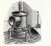
Fig. 12.—Girard-turbine with vertical shaft for medium falls.
