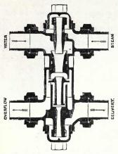
Fig. 101.—Gresham's automatic re-starting injector.
