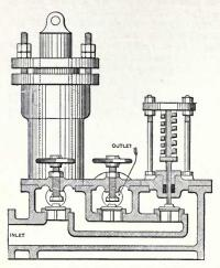
Fig. 194.-Vertical pump, with escape-valve.
