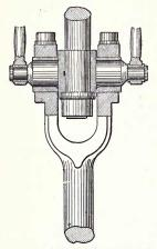
Fig. 268. Fork-end of a connecting-rod.
