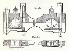
Figs. 282 and 283 .- Locomotive-engine side-rods.
