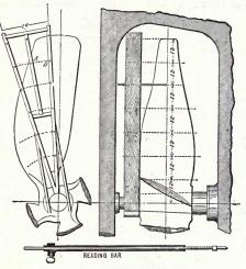
Fig. 315 .- Pitchometer for screw-propellers.
