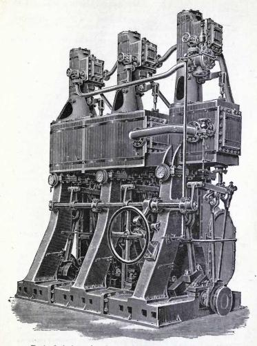
Fig. 369.—Quadruple-expansion surface-condensing marine-engines, by Rankin and Blackmore, Greenock
