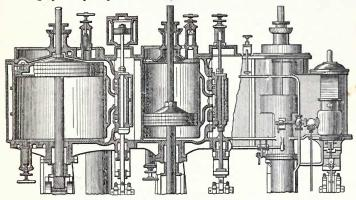
Fig. 326.- Cylinders of a set of triple-expansion marine-engines.
