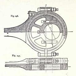
Figs. 246 and 247 .- Eccentrics and eccentric-straps of a locomotive-engine.
