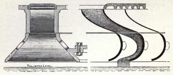
Figs. 10 and 11.-Sections of ports and buckets of the Girard-turbine.
