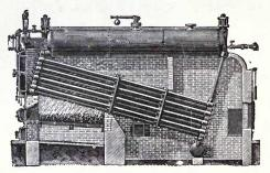
Fig. 130 .- Babcock and Wilcox water-tube boiler.
