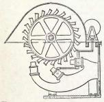
Fig. 14D.—Pelton Water-wheel with multiple nozzles. By the Pelton Water-wheel Co., San Francisco.
