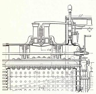
Fig. 66.-Fire-box of a locomotive-boiler.
