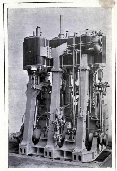
TRIPLE-EXPANSION MARINE-ENGINES OF 1200 I H.P. By Palmer & Co., Limited, Jarrow-on-Tyne.
