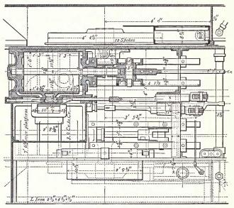
Fig. 324 .- Plan of the cylinders of a locomotive-engine.
