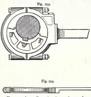
Figs. 253 and 254.—Eccentric and eccentric-strap of a stationary-engine.
