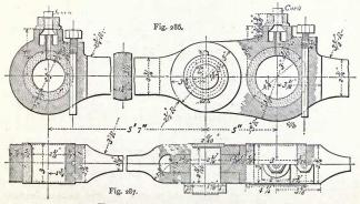
Figs. 285 and 287 .- Locomotive-engine side-rods.
