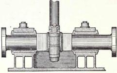
Fig. 288 .- Crank-shaft of a marine-engine.
