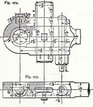
Figs. 274 and 275.—Small end of the connecting-rod of a locomotive-engine.
