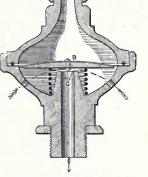
Fig. 173.—Air-valve for cor densing-engines.
