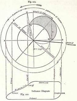
Figs. 210 and 211 .- Diagram of a slide-valve.
