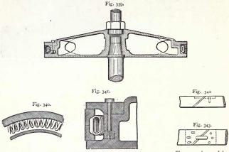
Figs. 342 an 1 343. — Joints of piston-rings.
