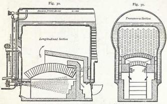
Figs. 30 and 31 .- Combustion-chamber for liquid-fuel.
