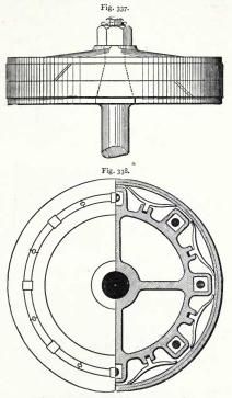
Figs. 337 and 338 .- Piston with adjustable rings.
