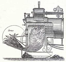
Fig. 46.-Ruston's straw-burning apparatus.
