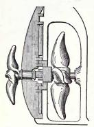
Fig. 316.-Kunstadter's screw-steering propeller, or rudder-screw.
