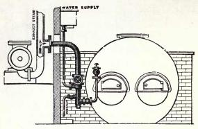
Fig. 103.-Method of fixing the exhaust-steam injector.
