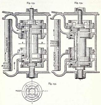
Figs. 233-235 .- Thom's piston-valves applied to a marine-engine.
