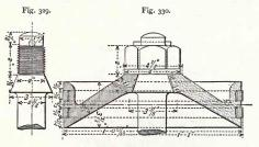
Figs. 329 and 330 .- Piston of a locomotive-engine.
