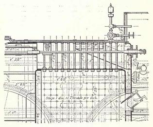
Fig. 65.-Fire-box of a locomotive-boiler.
