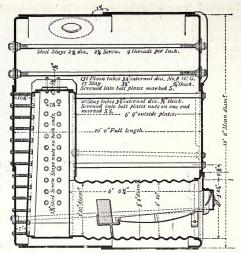
Fig. 124 .- Longitudinal section of a single-ended marine boiler, by Mr. J. Dickenson, Sunderland.
