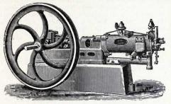
Fig. 17 .- " Otto " horizontal gas-engine.
