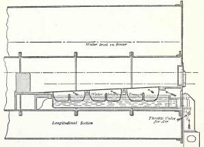
Figs. 47 and 48 .- Perrett's furnace for burning dust-fuel.
