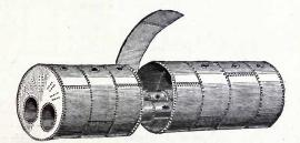
Fig. 153.-Explosion of a Lancashire-boiler from external corrosion, due to improper setting.
