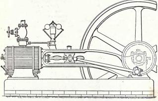
Fig. 362 .- Horizontal stationary non-condensing engine.
