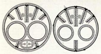
Fig. 100.—Section showing the front end-plate and gusset-stays of a Lancashire boiler.
