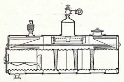
Fig. 107 .- Cornish boiler, with corrugated furnace-tube, fitted with Galloway-tubes.
