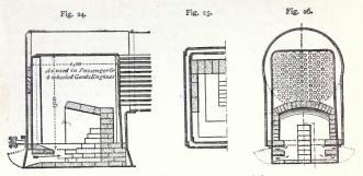
Figs. 24-26 .- Combustion-chamber for liquid-fuel.
