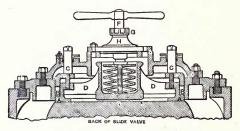
Fig. 221.-Claparede's balanced slide-valve.
