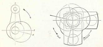
Fig. 198.-Crank and eccentric.
