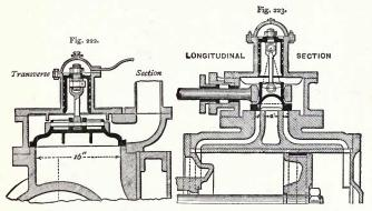
Figs. 222 and 223 .- Urquhart's balanced slide-valve applied to a locomotive-engine.
