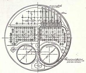
Fig. 128.—Half-end view and cross section of the boiler shown in Fig. 127.
