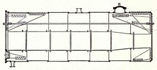
Fig. 108.-Longitudinal section of a Lancashire boiler.
