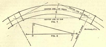
Put sin  $\phi = \frac{\frac{1}{2}L}{R}$ , in which L = length center to center of bolsters and R = radius of
