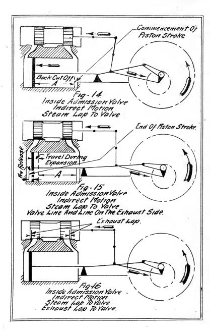
cylinder when the valve is on the point of "Cut Off," by virtue of which, the Piston is moved until the Valve arrives at the point of release, thus increasing its own volume at a reduced pressure.
