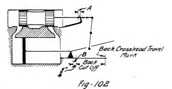
Compare this back Cut Off with the Front Cut Off and if equal the Cut Offs are O.K.
