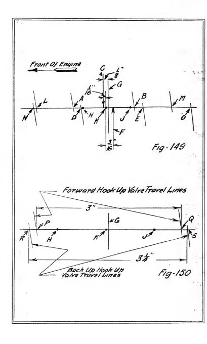
If we consider an inside admission value the motion is direct in forward gear which means the eccentric rod would have to be lengthened in our example.
