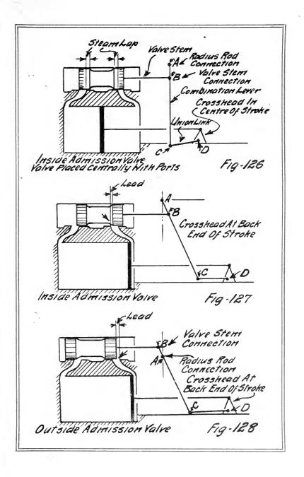
of the "short travel" and the "long travel" of valve is made when the combination lever is connected to the radius rod, see Figure 130.
