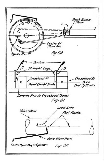
All dead centres can be found with the use of a tram in this manner and can be relied upon, providing the crosshead is moved to the end of its travel, the position of which corresponds with the dead centre being found and the line through centre of crosshead wrist pin being scribed to suit each dead centre as before detailed in the example just given.
