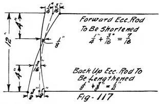
Determine the link lifter length adjustment required to equalize the hook up valve travels last figured. The forward  $2\frac{1}{2}''$  and the back up  $2\frac{3}{4}''$  will both equal
