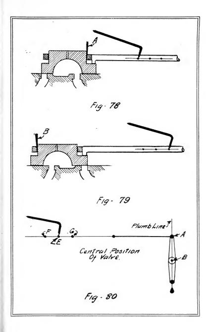
being in no way connected to the side of the boiler. The reverse lever in mid gear notch should stand plumb, when main frames are levelled, see "A," Figure 81. When reverse lever is placed in the middle notch of its rack
