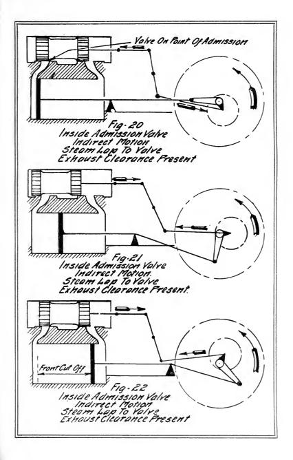
the exhaust sides of the valve We now have, see Figure 18, what is known as "Exhaust Clearance," i.e., the distance between the edge of valve on the exhaust side and the nearest edge of steam port when valve is placed on the centre of its seat. When exhaust clearance is arranged it has the opposite effect to exhaust lap, i.e., release occurs earlier during the stroke of the piston and "Pre-release" is lengthened.
