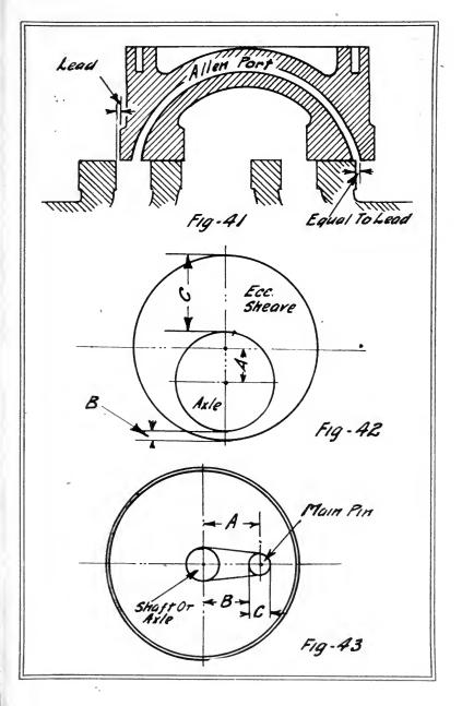
the further movement of the piston compresses same until the point of Admission is reached, which again allows of the entry of live boiler steam. This operation occurs at both ends of cylinder and is continuous whilst engine remains in service.
