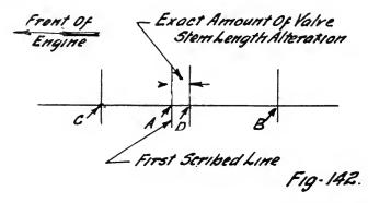
Place tram point in centre of link foot pin again, and with other tram point, scribe another arc "B" to cut the straight line "F." The distance between "A" and "B" is the amount of alteration to make in the length of eccentric rod. To bring the first arc to the second means shortening the eccentric rod in this case.
