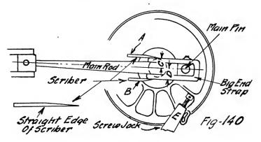
Measure the distance "C" to see if it equals the distance "D." If not, apply a jack (to slip the driving wheels) as shown at "E" until "C" equals "D," both being measured from the centre of driving axle.
