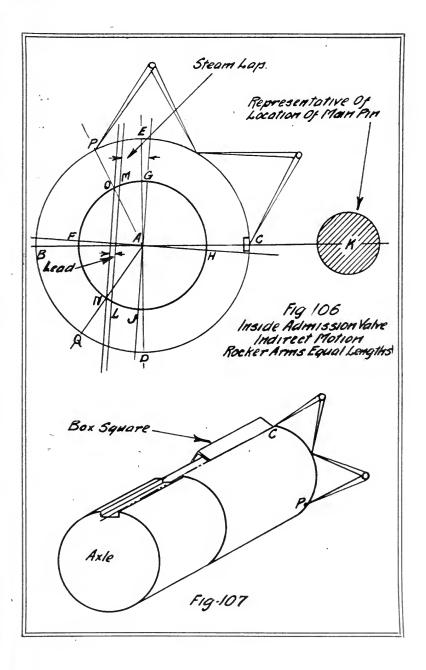
centre line of motion lies at an angle generally to the line "A.K," which passes through the centre of axle and the centre of main pin.
