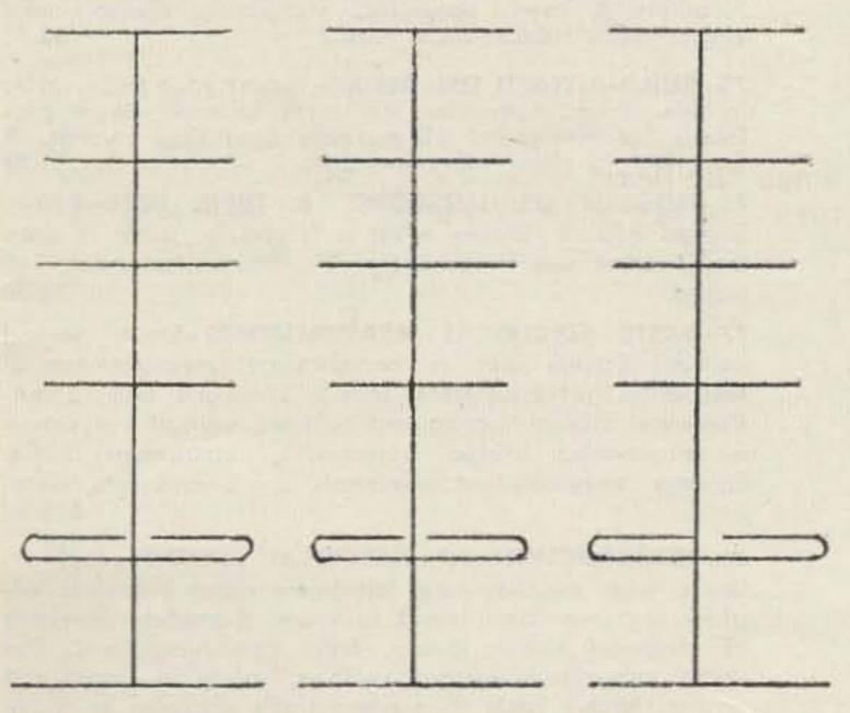
balun on 2 meters, which will of course be a proper match on both bands. It must be mentioned here that the placement of the antenna, particularly in the height above ground and other objects will to some extent affect the gain and impedance characteristics of the beam on both bands.
