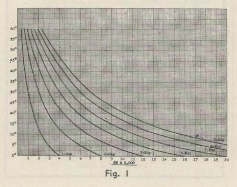
you that radiation angles for DX propagation should be around 15° or less, to be practical. For example: the path New York to Alaska is 5,400 Km and from the chart the smallest number of hops is 2-Hops with a radiation angle of about 7°. If 3-Hops occur, the radiation angle will be about 15°. In general we find DX propagation having angles of departure and arrival from 2° to 5° to 10° and 12°
