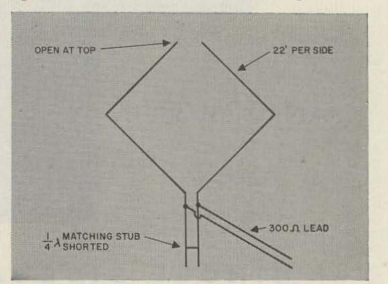
Fig. I. Bi-square antenna for 15 meters. A horizontally polarized, broadside, bi-directional array with a gain of about 4 db. It is constructed with ordinary antenna wire and fed with twinlead. It requires only one 35 foot (or taller) pole for support.
