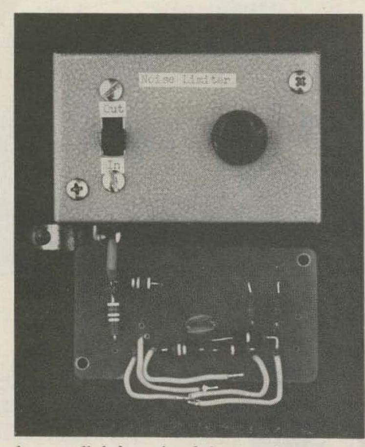
down well below signal level and even performed as well as the TNS limiter in the Pontiac except for the squelch action. A printed circuit board was then constructed and components were transferred from the phenolic board.
