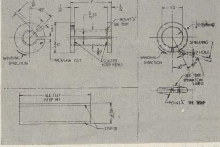
C13—Shield PSIA, Mat'l .005 Brass or Copper C12—Primary bobbin PSI, Mat'l Brass or Copper C14—Shield PS2, Mat'l copper
