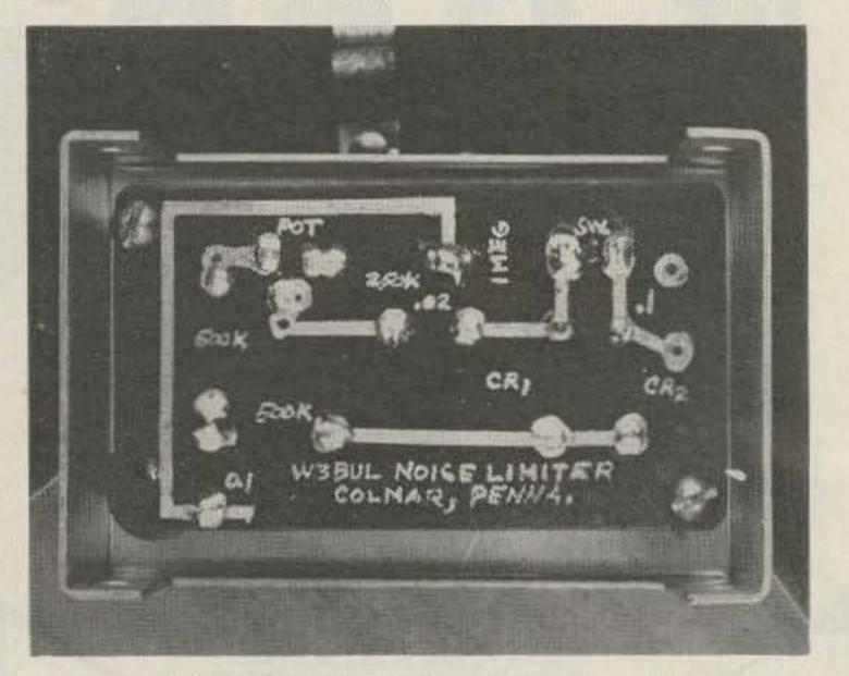
and drill 1/16 inch holes for mounting component parts. Mount components as shown in Fig. 4 and solder in place using a good rosin core solder.
