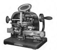
FIG. 88.—Emboasing machine; hand "Graphotype"; Addressograph. To face page 101.]
