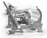
FIG. 475.-Casting-press for semicy/indrical plates; opened for trimming and removing the plate. PLATE XCVI.
