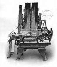
FIG. 343.-Dow composing and line-justifying machine; front view. [To face page 364
