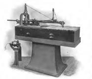
FIG. 164.-Barr or Linotype direct-cutting panlograph for formors.
