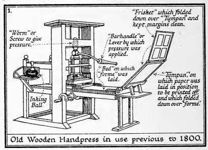
reverse from solid panels of wood) was inked over with an ink ball or ink pad of leather: the paper laid carefully upon it; and pressed down by means of a screw much as an old-fashioned linen press or a letter-copying
