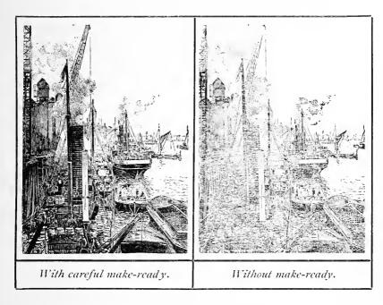
The difference will be best seen in the stippled smoke, where the dots of the stipple are as close together as in a coarse-screened half-tone plate.
