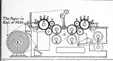
Diagram showing main features of a Rotary Press.
