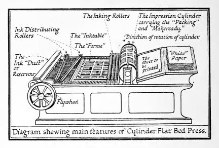
B. With printing surface flat, and moving back and forth, the paper applied by revolving cylinder (König circa 1811). They are called flat-bed cylinder machines. The development is one of speed, and size of forme and paper that can be handled.
