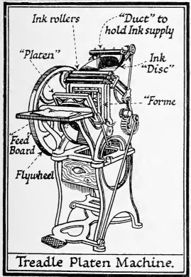
presses. Here the paper is laid on a flat bed (the platen), the platen is raised, carries the paper to the inked forme and lowers itself again to allow the machineminder to take off the printed copy and lay a new sheet. This form of machine is used for smaller work whether from type or plates in monochrome colour.
