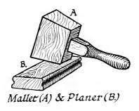
[The matter in the forme is levelled by the compositor with mallet and planer.]
