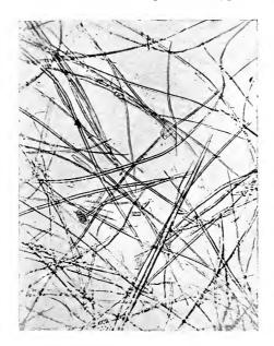
FIG. 6. ESPARTO FIBRES AND CELLS
