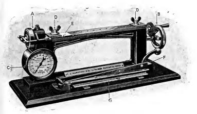
FIG. 26. MARSHALL'S PAPER-TESTING MACHINE
