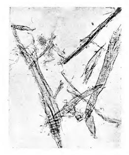
FIG. 9. MECHANICAL WOOD-PULP FIBRES
