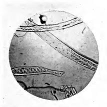
FIG. 8. PITTED VESSELS ON CHEMICAL WOOD
