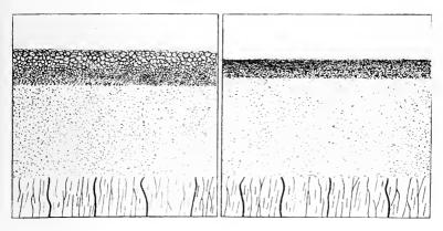
$$\operatorname{Fig.~XIV}$$  Showing the Effect of a Rain in Settling a Soil Mulch
