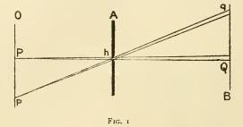
to produce any developable effect on a sensitive plate, but it has the virtue of always drawing form correctly and in true perspective. Fig. 1 shows that all the little beams of light that reach the image screen must pass through the pin-hole and intersect one another at the point h, and, this being
