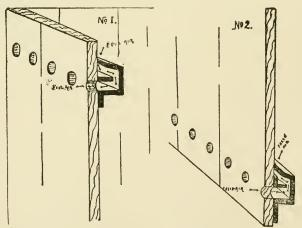
Illustration Nos. 1 and 2 Simple Method of Ventilating a Dark Room See Paragraph No. 11
