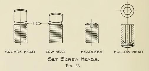
are no projecting parts to catch the clothing. It has the objection, however, that one side is apt to break off. To remedy this defect, a hollow head set screw has been designed. This requires a special wrench bent from a hexagon steel bar.
