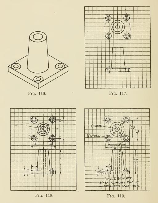
Dimensions should always be given from center lines and finished surfaces. When a circle is to be drawn, the radius should be pointed off each way on the center lines from the point where the two center lines cross. Through the four points thus located, a circle may readily be passed freehand. Always put a complete
