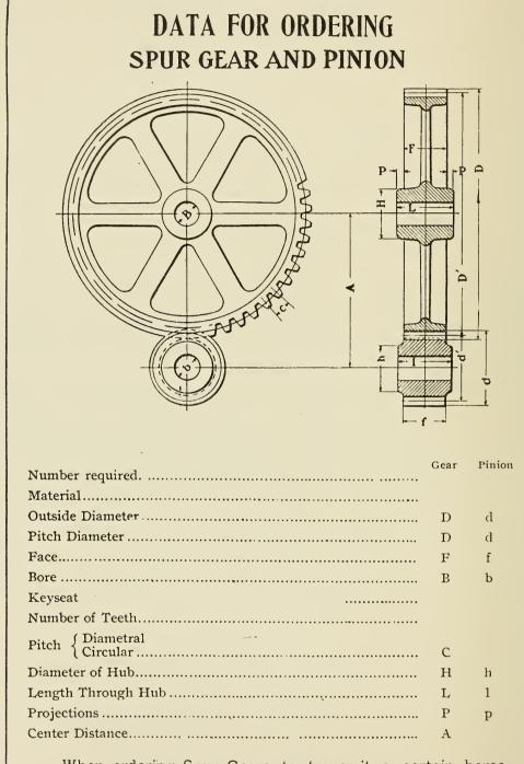
When ordering Spur Gears to transmit a certain horsepower, do not fail to state number of revolutions, size of bores, and largest and smallest permissible diameters.
