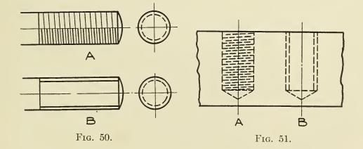
other conventions that are occasionally seen. The convention at B in these figures is especially simple and convenient for sketching purposes but has the great disadvantage that it bears no resemblance to screw threads and hence is not recommended.
