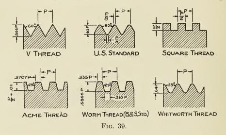
stronger bolt than if the V thread were used. It is used generally for bolts, studs and cap screws. The width of the flat surface at the top and bottom of the threads is one-eighth of the pitch.
