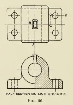
along the lines ABCDE in the upper plan so as to show the interior construction at the oil hole and also at a bolt hole.
