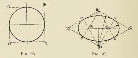
Suppose we wish to represent a 1-in. circle on the top isometric plane; see Figs. 96 and 97. We first imagine that the circle is enclosed by a 1-in. square ABCD, Fig. 97, being sure to get the sides of this square parallel to the proper isometric axes. After the square is outlined, we draw the diagonals of this square, AC and BD. Then we connect the middle points of AB and BC with D, getting the lines MD and ND. In the same manner,
