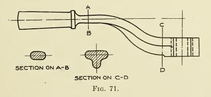
section is shown as if it passed just to one side of the arms. As stated in Article 38, it is the general practice not to cross-hatch the arms of pulleys, hand wheels, etc., when cut lengthwise. Only the hub and rim should be cross-hatched. It should be noted that the inside surfaces of the rim should be shown by full object lines all the way across, as if the section plane had been passed just in front of the arms, thus showing only the rim and hub in section. SHOP SKETCHING
