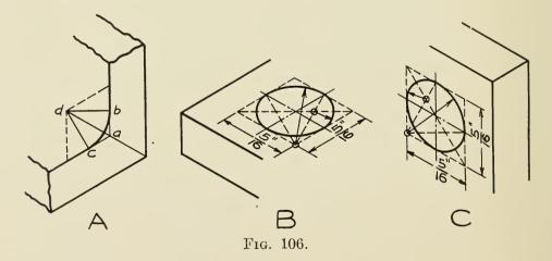
first drawing circumscribing squares whose sides make angles of  $30^{\circ}$  with the horizontal. The method of constructing these rivet holes and the  $\frac{3}{16}$ -in. fillet is shown in the enlarged views of Fig. 106. Note that the holes appear different in the horizontal and
