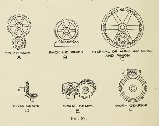
the other is called the *driver*; the other one is called the *driven* gear or the follower. The change gears of a lathe are good examples of spur gears.
