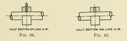
with the set screw in place. Fig. 65 shows the same collar with the set screw removed, and the tapped hole which receives it exposed to view.
