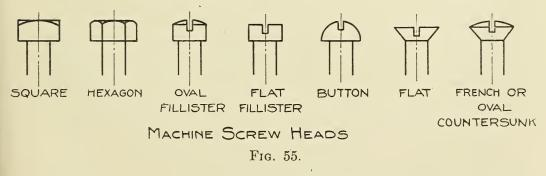
which a wrench can be used. These heads are usually thicker and of smaller diameter than the U. S. standard bolt heads. All of the other heads are provided with slots for a screw driver.
