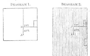
If you cannot find any break in the tin, follow the dotted line "A" "B" to the upper edge of the roof, watching carefully. If you can still find no break in the tin, notice if there is a joint close to the mark "A," and
