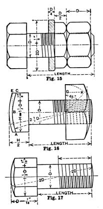
corners, as in Figs. 12 and 14, describe A B C tangent to top with radius equal to diameter of bolt. From the same center describe arc E F, point F being equal in height to C.
