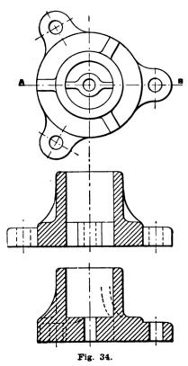
acter, like that of the Check Valve, PLATE 2, it is common to draw the lines which are visible beyond the section.
