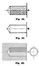
the threads will be inclined in the opposite direction to that of Fig. 24.
