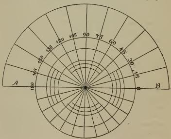
The centre of the lens must be exactly over the centre of the circle, and the horizontal line marked on the lens from nose to temple must cover the horizontal line AB. We now observe in what direction the ink-mark points, and we have the degree of the cyl. axis. In making this proof we must hold always the outside of the lens upwards, not towards the paper.
