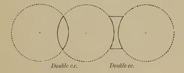
Periscopic ex or ee, the two curves are formed by spheres of different sizes.
