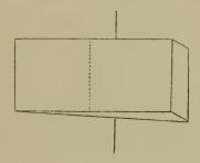
The thicker end of the prism is called the base; and base in "means to place the thicker end towards the nose-piece of frame. In setting such lenses, care should be taken that a straight line is not broken in either of the lenses.
