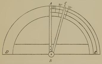
The joint B must be exactly in the centre of that semicircle DAE. That side of the rivetted or stationary bar AB which is nearest E, is precisely 90° from either D or E. The arm BC is movable, and indicates the numbers of degrees of a prism placed in the opening A B C. I present also another easy way of testing prisms by the use of a simple ruler.
