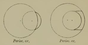
Plane ex or ec, formed by a plane and one sphere. The plane is either inside or outside of the sphere.
