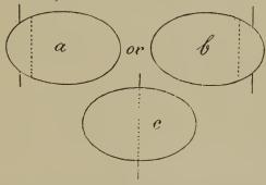
Now, move your lens slowly towards the centre till you find the line unbroken (Fig. c); mark this line with ink, and it will be the optic line of the lens in one direction; but you have not yet determined the optic centre. Now turn the lens in your hand  $90^{\circ}$ , so that the line on the paper and the mark on the lens form a right angle.
