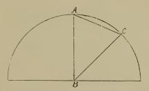
With a "trial box," containing test prisms, the strength of one lens may be determined by neutralizing it by another, as I have shown before; but to ascertain also the correctness of your test-prisms, it is necessary to construct a tool made of a protractor, like the following.
