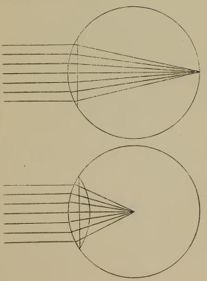
The lens of the first figure is plano-convex, and its focus is at the end of the diameter: it is cx No. 2 (two inch focus). The lens of the second figure is double cx, and its focus is at the end of the radius, or at the centre; its strength is + 1 (one inch focus).
