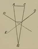
A B C is a prism, D is a ray of light falling on it, and is bent off in the direction of O. If our eye is placed at O, we see the object D, from which the light is emitted, in the direction of O E; and although the ray of light is bent towards the base of the prism, it comes apparently from the thinner part of it.
