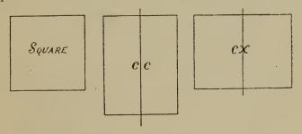
A cx cyl. lens with axis vertical will lengthen the horizontal sides, producing a horizontal parallelogram. A cc cyl. lens will have the same effect, with the difference that the lengthening is in the direction of the axis, and if this is vertical, the parallelogram will be vertical. This ex-
