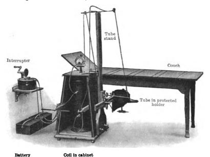
Fig. 83.—Portable X-ray installation arranged for radiography from beneath couch.
