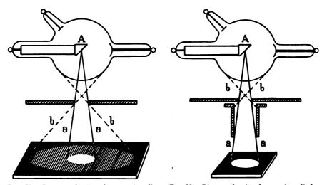
Fig. 52.—Diagram showing the use of a diaphragm between tube and plate. (Schall.)
