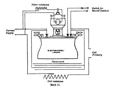
Fig. 13.—Plan of connections for Dreadnought interrupter.
