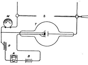
Fig. 35.—Diagram of connections for Coolidge tube.
