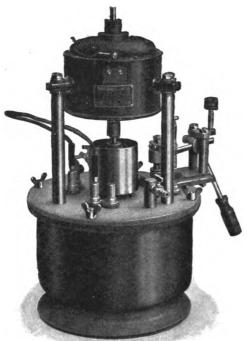
Fig. 189.—Mercury interrupter with gas di-electric. (Schall.)
