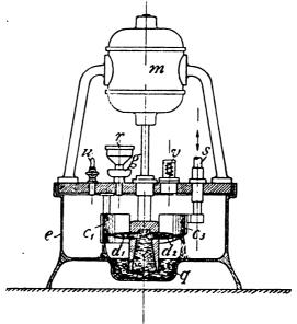
mercury never becomes Fig. 12.—Diagram to illustrate construction of a centrifugal mercury interrupter. (Siemens.)
