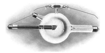
Fig. 42.—Gundelach tube with regenerator. (Siemens.) a, wire. b, wire. c, metal cap. d, metal cap.
