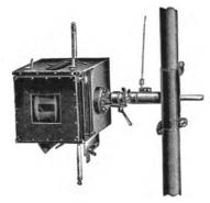
Fig. 65.—Tube-box with rectangular diaphragm.
