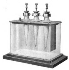
Fig. 20.—Three-point electrolytic interrupter. (Siemens.)
