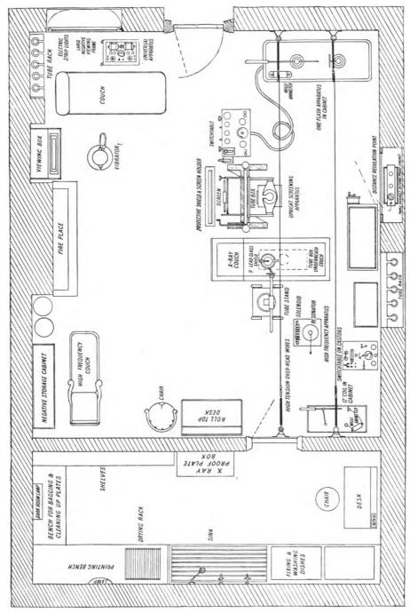
The equipment is arranged for radiographic and therapeutic work, and includes accessory apparatus, high frequency, galvanism and faradism, vibrator, etc. Fig. 80.—Plan for consulting-room or hospital outfit, showing method of arranging apparatus in order to facilitate rapid working.
