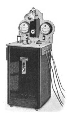
Fig. 22.—Trolley control table, with resistances arranged to facilitate time and rapid exposures. (Siemens.)
