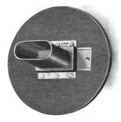
Fig. 56.—Walter's radiometer. (Siemens.)
