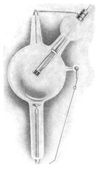
Fig. 28.—Water-cooled tube arranged for overhead work. (C. Andrews.)
