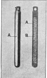
Fig. 230.—The length of the tube is determined by the diameter and the smallest space the radium can be packed into.
