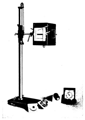
Fig. 61.—Pillar stand, protected tube-box and accessories. (Siemens.)
