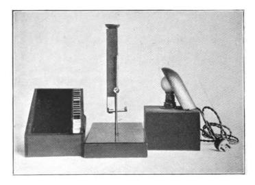
Fig. 210.—Loviboud's tintometer, adapted and standardised for the accurate measurement of the colour-changes in the Sabouraud-Noiré pastille by Dr. Dudley Corbett. (The Tintometer, Ltd.)
