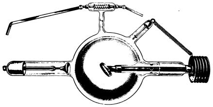
Fig. 26.—Radiator tube constructed for heavy discharges. (Cossar.)
