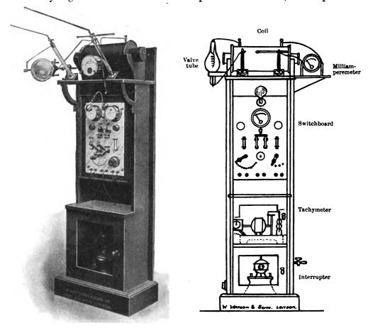
Fig. 199.—Apparatus arranged on an upright cabinet. Fig. 200.—Diagram to show arrangement of apparatus on an upright cabinet.
