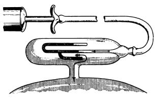
Fig. 41.—Bauer air-valve. (Favre.)
