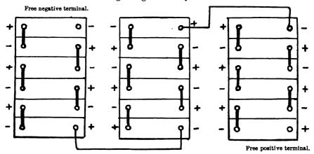
Fig. 6.—Accumulator connections. The positive wire going to the coil is connected up with the free positive terminal of the accumulators and the negative wire with the free negative terminal.
