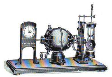
Fig. 191.—Dipping interrupter with revolution counter or tachymeter.
