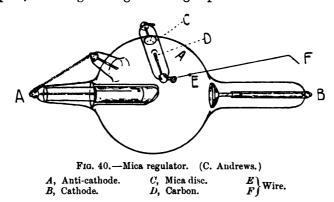
the current should be passed through the regulator depends obviously upon the degree of hardness of the tube, and the amount of softening which it is desired to attain; but in any case it is wiser to switch off the current as soon as the fiery appearance is seen in the mica, swing back the regulator wire, and test the tube; and then to repeat the process of regulation if necessary.
