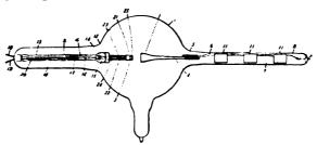
Fig. 33.—Diagram of Coolidge tube.
