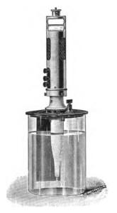
Fig. 21.—Single-point electrolytic interrupter. (Watson.) The upper part of the interrupter has attached to it a solenoid which is connected electrically to the switch-table, allowing of the control of the depth of point in the fluid.
