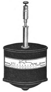
proportion to the electrical tension in the secondary circuit, and is indicated by the deviation of a pointer over a suitably divided scale.
