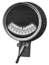
Fig. 186.—Milliamperemeter. (Siemens.)
