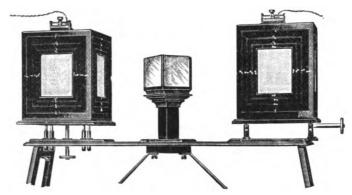
Fig. 89.—Wheatstone stereoscope. (Watson.
