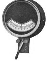
Fig. 60.—Milliamperemeter. (Siemens.)
