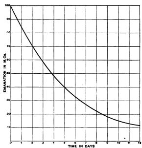
The same fraction, how- Fig. 224.—Curve showing decay of radium emanation with time.
