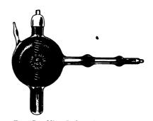
Fig. 47.—Oliver Lodge valve tube. (Cossar.)
