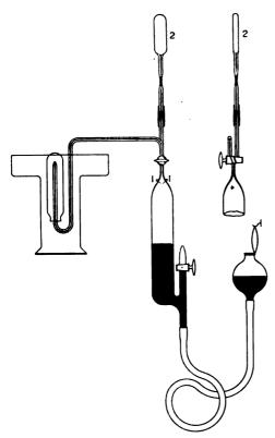
Fig. 223.—Apparatus for charging glass or other applicators with radium emanation after sparking.
