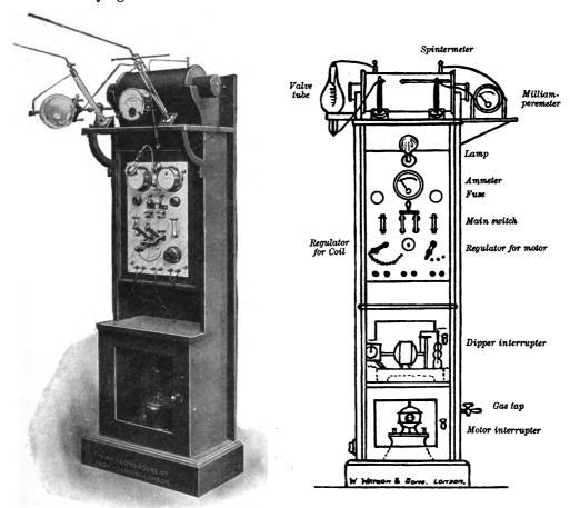
Fig. 78.— Aconvenient form of apparatus arranged on an upright cabinet. (Watson.)
