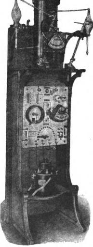
Fig. 1.—Gaiffe Rochefort outfit for alternating or continuous current. For alternating supply there is a difference in the arrangement of the interrupter. (Medical Supply Association.)
