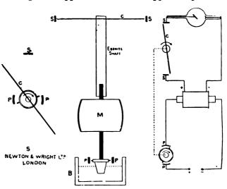
Fig. 193.—Diagram of connections for Morton rectifier.
