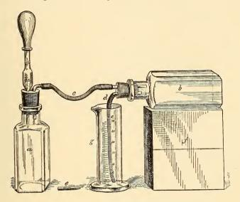
Fig. 4.-Squibb's urea apparatus, for the approximate estimation of urea in urine.
