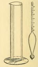
Fig. 2.—Urinometer and urinometer-glass (slightly smaller than one-half actual size).
