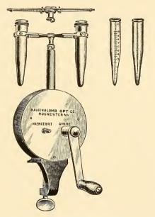
Fig. 23.—The Bausch and Lomb spiral-gear urinary centrifuge with tubes (one-fourth actual size).
