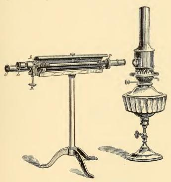
Fig. 18.—The Schmidt & Haensch polariscope.
