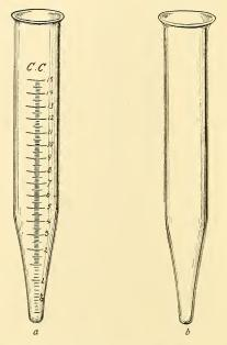
Fig. 22.—Tubes for the Purdy centrifuge: a, Percentage tube; b, sediment tube.
