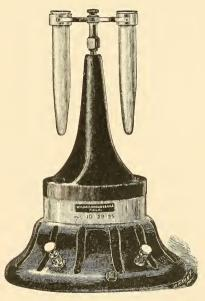
Fig. 21.—The Purdy electric centrifuge.
