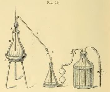
Apparatus for the determination of nitrogen., (Simon.)
