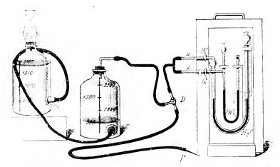
Fig. 151. (Diagram showing the action of the Brauer apparatus, (Sauerbruch,)
