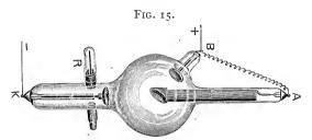
Gundelach tube with heavy anode for radiographic work.
