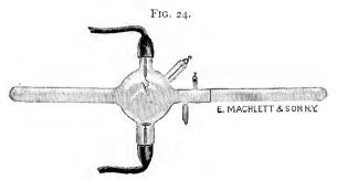
Tube made of lead glass for the treatment of cavities.
