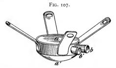
a. Rock-crystal lens. The projections b and b' are for attaching water-cooling tube and outflow.
