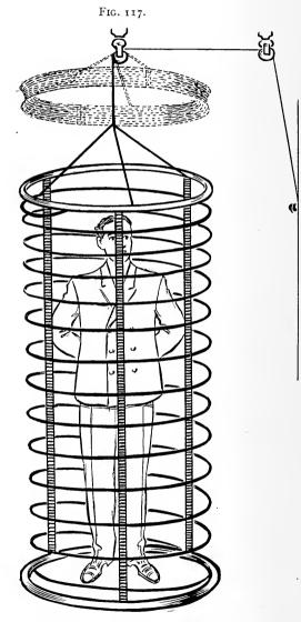
Cage solenoid for autocondensation.
