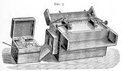
Portable coil to be attached to street current.
