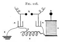
Showing connections for resonator.
