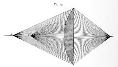
Illustrating the different foci of chemical rays (V) and the heat-producing rays (R).
