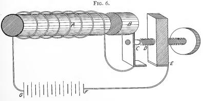
Showing detail construction of primary coil, with vibratory interrupter.
