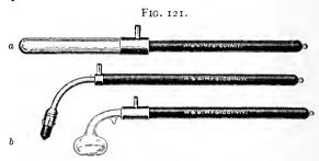
Vacuum electrodes: *a*, glass cone filled with metal filings coated with silver upon the inner surface; *b*, carbon point for single spark.
