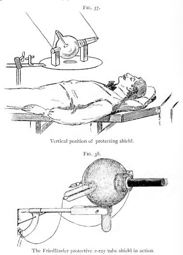
In Fig. 38 is shown a hood-like tube-holder which carries out my original idea of a funnel to include the tube as one piece in a very practical way. The manufacturers, Messrs. Friedländer & Co., have kindly placed
