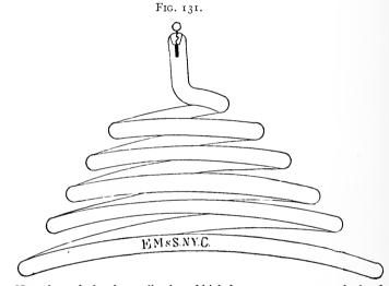
New electrode for the application of high-frequency currents to the head.
