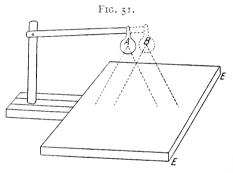
.4. Crookes' tube in position for first exposure. B. Crookes' tube in position for second exposure. E. E. Plate-holder.
