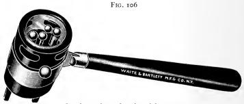
Spark-gap lamp for ultraviolet rays.
