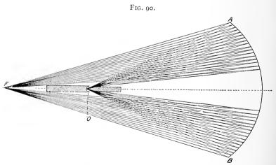
Illustrating loss of light for reflectors by the interposition of the carbons.
