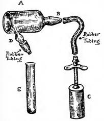
F16. 92b.—Suction apparatus for collecting blood for the Wassermann Reaction. A, suction glass connecting at B with suction pump  $C_i$ the blood flows through D connected by rubber stopper with an ordinary test tube, E.— Blackfan.
