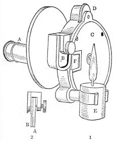
FIG. 97.—1. Dare's harmoglobinometer. A, telescope; B, pipette in place; C, case enclosing color-prism; D, milled head; C, case lendosing prism; E, candle; F, window admitting light to color-prism. 2. Pipette. A, the white glass; B, clear glass disk.—Emerson.
