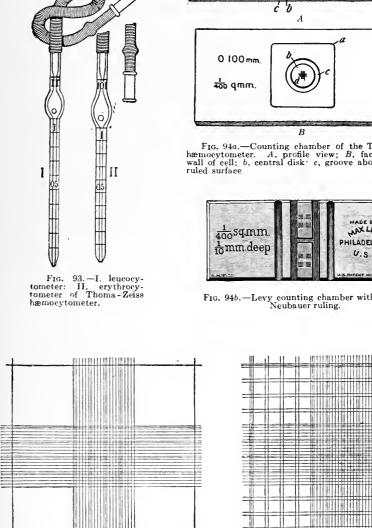
FIG. 94a.—Counting chamber of the Thoma-Zeiss hæmocytometer. A, profile view; B, face view; a, wall of cell; b, central disk c, groove about disk; d,
