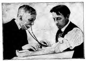
FIG. 71a.-Sanborn's sphygmomanometer. Auscultatory method.
