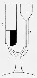
FIG. 29.—Horismascope. A, The arm of the U-shaped tube with fine bore; B, bulb in which HNO<sub>5</sub> is poured after the tubes are filled with urine; C, wide-bore arm for urine, with background.
