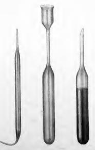
F1G. 122b.—Tubes used in serum work. The tube to the left is used to collect blood. The others for bacterium emulsions. (Reduced just one-half).
