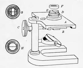
FIG. 105.—Miescher's modification of Fleischl's hæmogloblnometer. A, stage; B, color-prism rack; C, milled head; D, ceil; E, cover-glass; F, cap; G, cell seen from above; H, cell of Fleischl's instrument.
