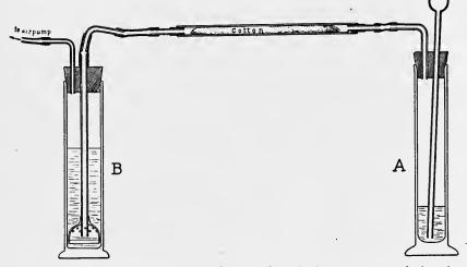
F1G. 23—Folin's apparatus for ammonia and acetone determination. A, narrow tube for urine, connected by a tube containing cotton, with B, the cylinder containing acid.
