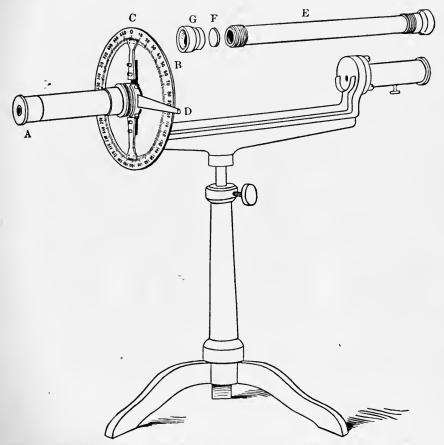
F1G. 25.—Half-shadow saccharometer. A, ocular used in focussing the field; B, graduated disk; C, vernier; D, lever for rotating analyzer; E, tube for urine; F, glass disk; and G, cap for end.
