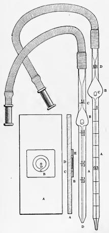
FIG.94.—Blood-counter (Thoma-Zeiss). To the right is the ordinary form of pipette for red cells; the other is a leucocyte pipette with improved markings and point, D. The ruled counting chamber is shown on edge and face view. A, the slide; B, the ring; D, the ruled table and C, the "ditch;" E, the cover-glass.
