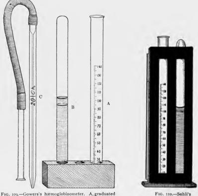
tube; B, color-tube; C, pipette.
