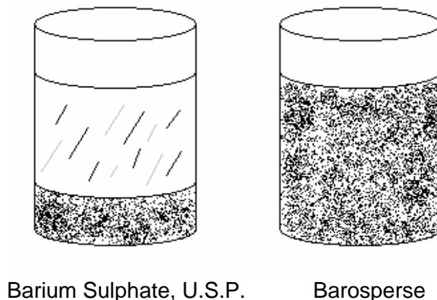
Figure 1-10. Comparison of Barium Sulphate, U.S.P., and Barospense after being stirred and resting a few minutes.
