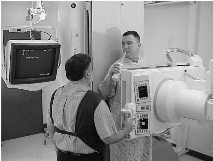
Figure 1-6. Image intensifier unit hooked up with an x-ray unit and in position for vertical fluoroscopy.
