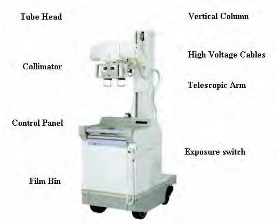
Figure 4-17: General Electric AMX 4, Portable radiographic equipment.
