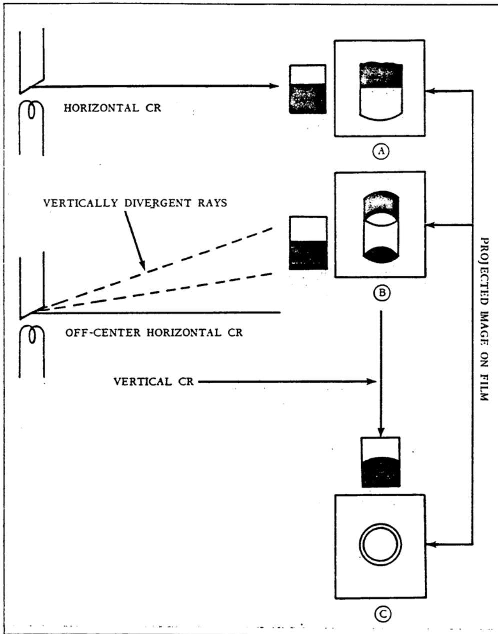
Figure 4-12. Schematic representation of fluid-level radiography with a drinking glass partially filled with barium sulfate suspension demonstrated in steps A, B and C.
