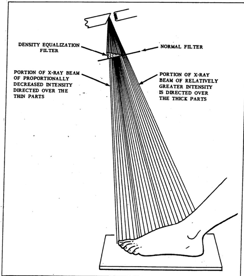
Figure 1-8. Relationships of the density equalization filter, the x-ray cone (or beam), and the thin and thick parts of the anatomical structure being radiographed.
