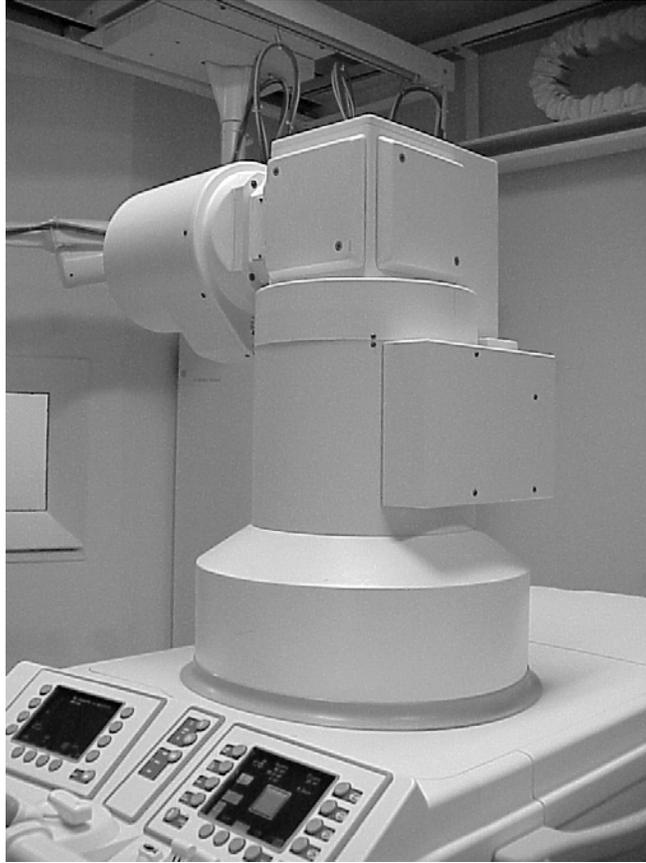
Figure 1-5. A typical x-ray image intensifier.
