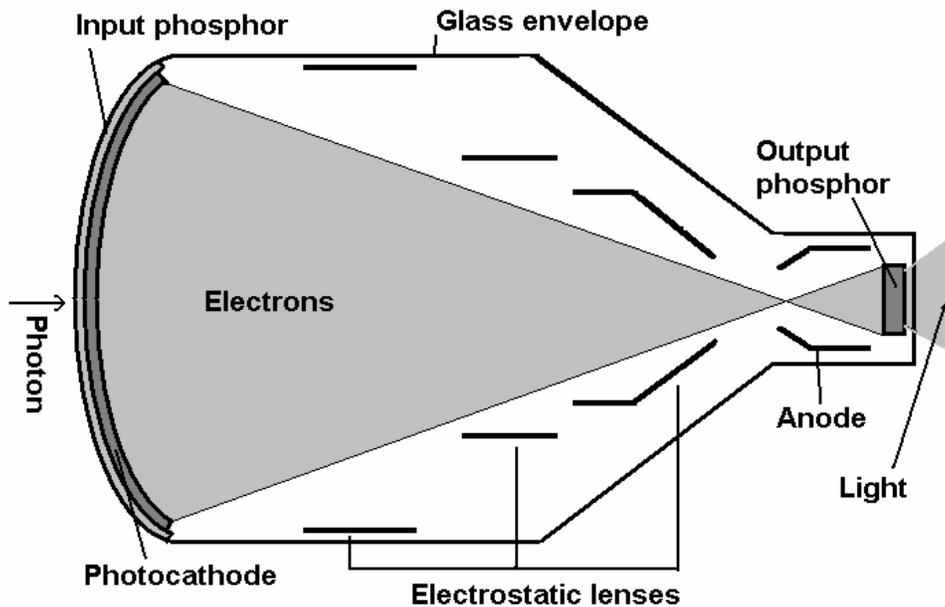
Figure 1-4. An image intensification tube.
