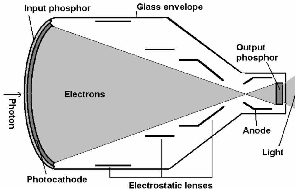
Figure 1-1. An image intensification tube.
