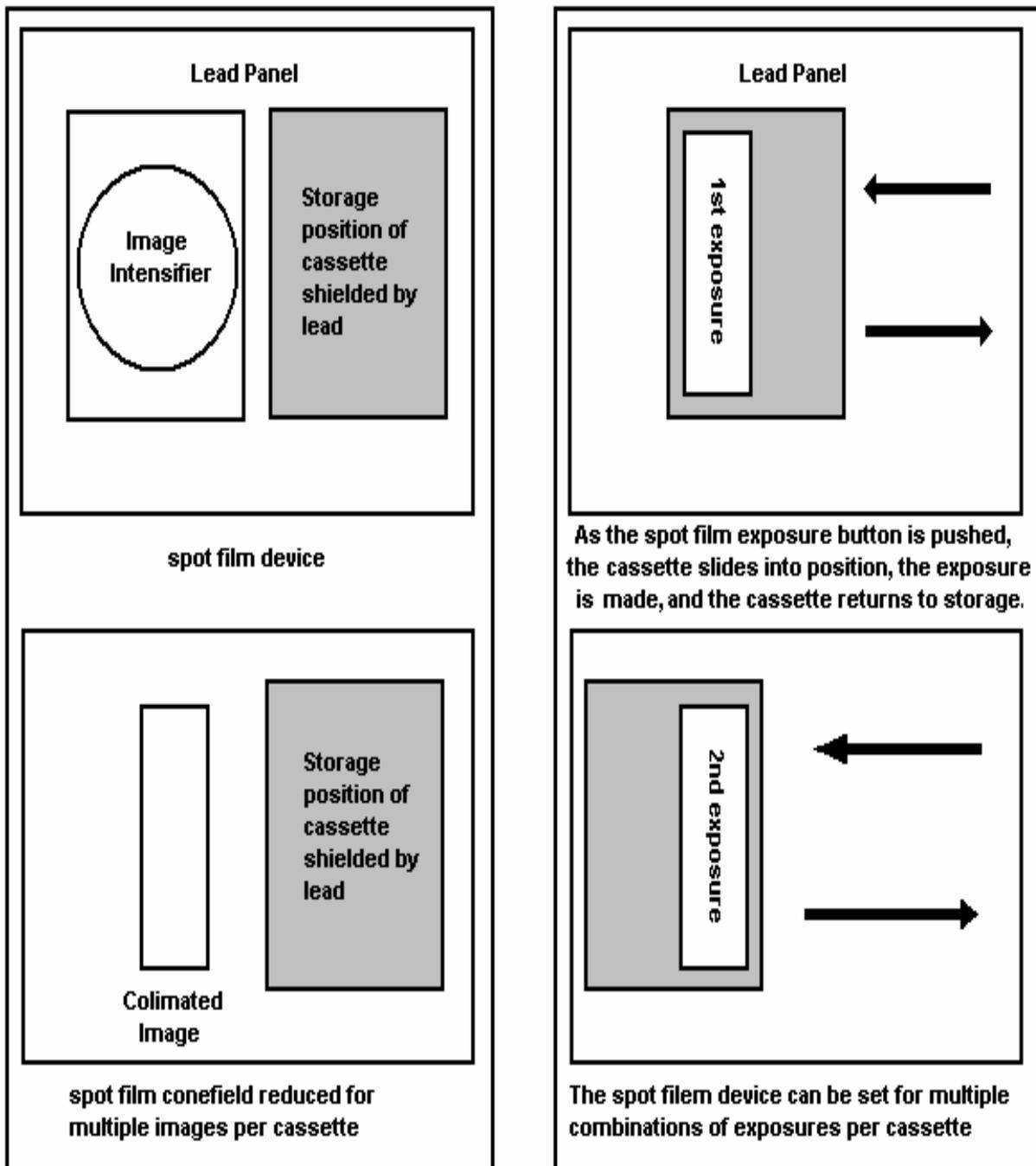
Figure 1-2. Spot-film radiography and serialography.
