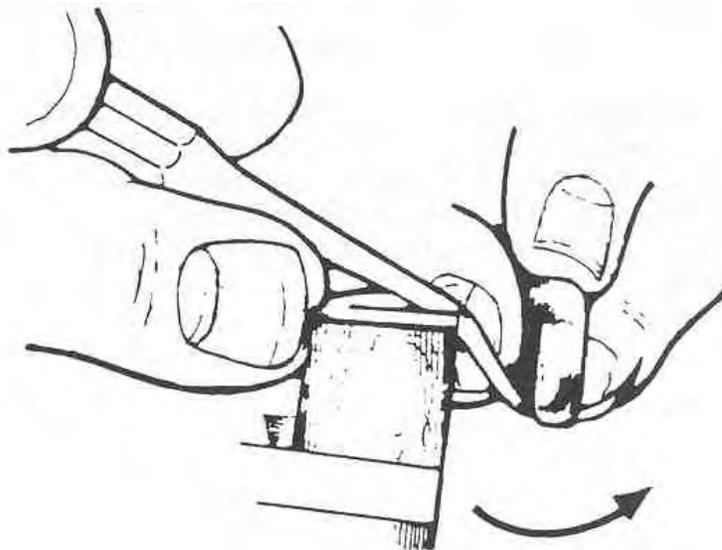
Figure 1-5. Sharpening an instrument using a hand stone.
