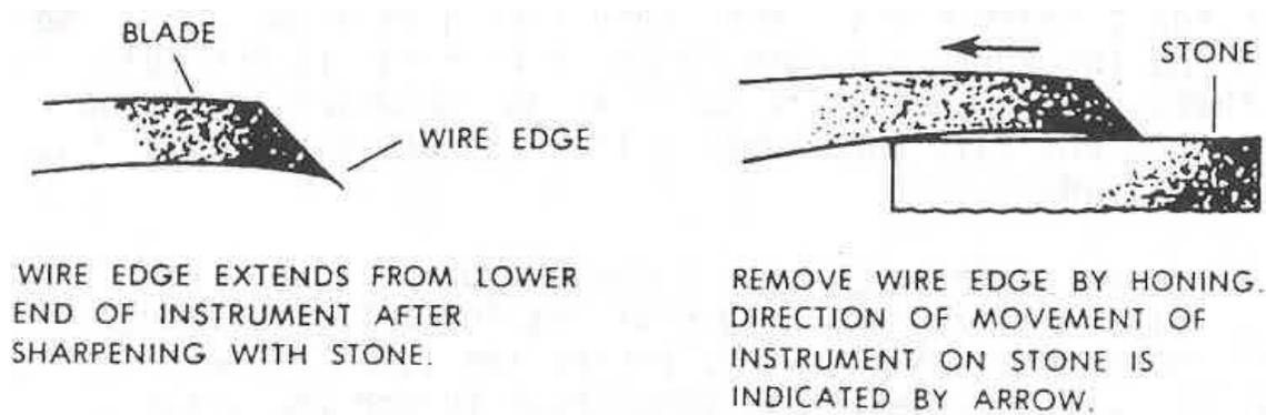
**NOTE:** Using a hand stone, the instrument should be stabilized while being sharpened. the instrument is placed so the inner concave surface is upward and parallel to the floor. The stone is placed on the inner surface of the blade at its junction with the shank and then moved back and forth in a sawing motion until it reaches the tip. The outer surface is honed slightly to remove the wire edge.
