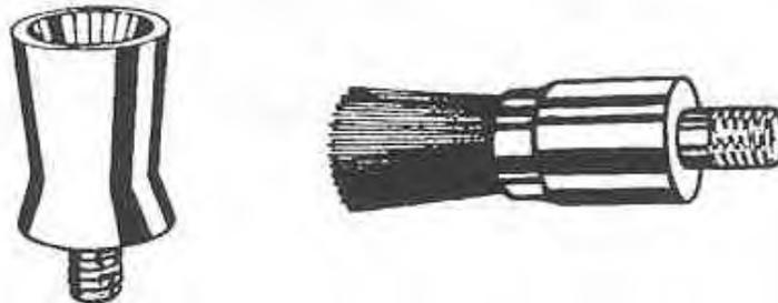
Figure 2-28. Polishing cup and polishing brush.
