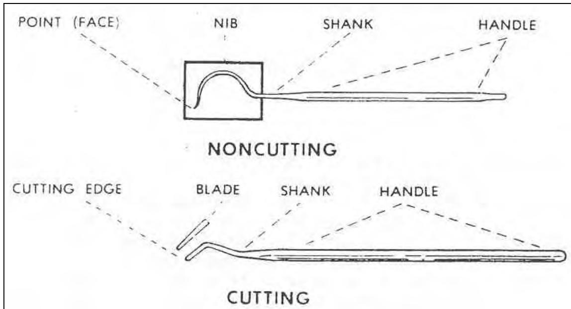
Figure 1-1. Parts of a hand instrument.
