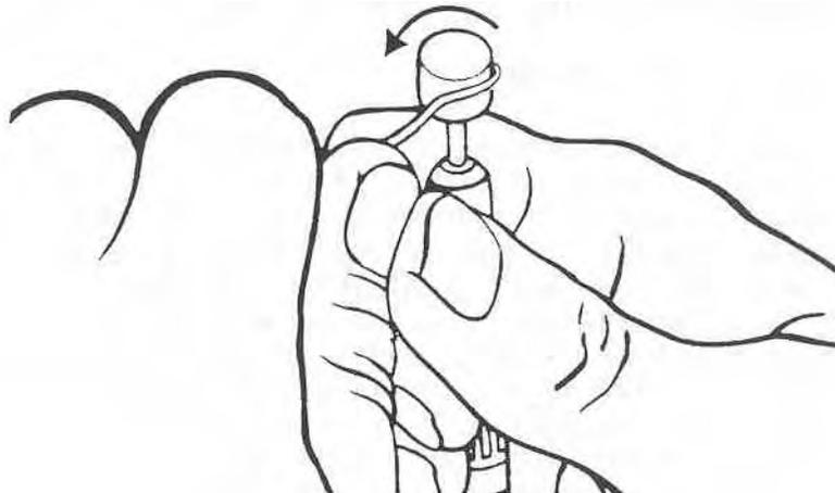
Figure 1-7. Sharpening an instrument using a mounted stone.
