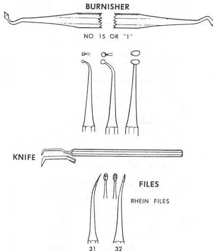
Figure 2-23. Hand finishing instruments.
