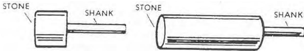
**NOTE:** Using a mounted stone, the instrument is held in a palm and thumb grasp, with the inner concave surface facing upward, and the tip toward the dental specialist. The stone is made to revolve slowly in the handpiece. Place the slowly revolving stone against the inner surface of the junction of the blade and the shank and draw it slowly toward the tip until it passes off the scaler. Both lateral edges will be sharpened simultaneously.
