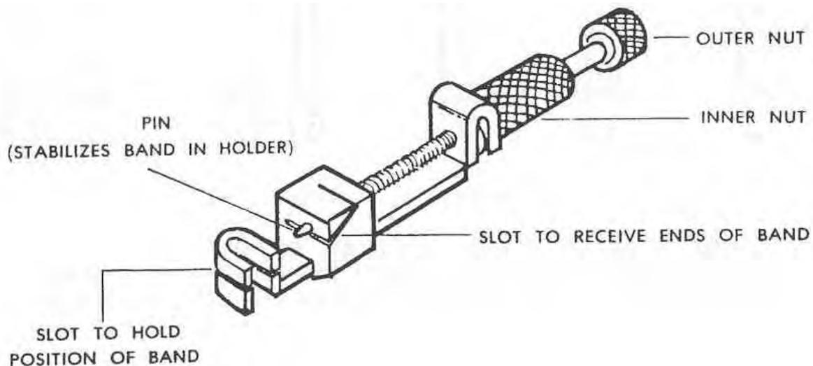
Figure 2-10. Tofflemire matrix retainer.
