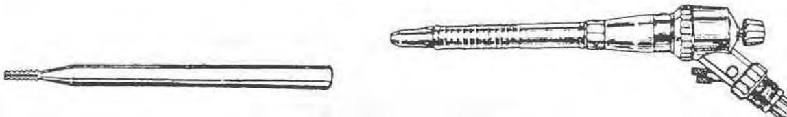
High speed handpiece (HSHP): Burs used in this handpiece will have a smooth shank like that of the straight handpiece, but the shank will be smaller and much shorter. These are known as "friction grip" burs.
