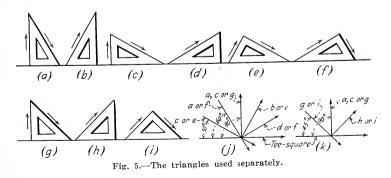
Lines parallel to any given line may be drawn conveniently by bringing one edge of a triangle to coincide with the line, and then placing
