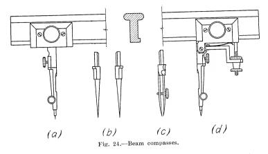
essentially of a bar or beam on which may be clamped suitable attachments for holding the needle point and the pen or pencil points. The pen point (c) replaces the pencil point (d) in inking; and all these points, including the divider points (b), are interchangeable. A serviceable beam compass of cheaper construction is shown in Fig. 25.
