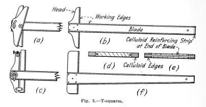
Either an extra swivel head (Fig. 3a) or an adjustable blade (Fig. 3c) are convenient in work involving many parallel lines at odd angles. The micrometer screw in the head of the latter style offers a convenient means of trueing up the blade to agree with the drawing.
