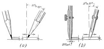
Fig. 10 .- Ruling positions for drawing pencil and pen.
