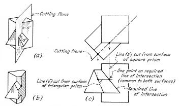
Fig. 62 .- Method of finding points on the line of intersection of two surfaces.
