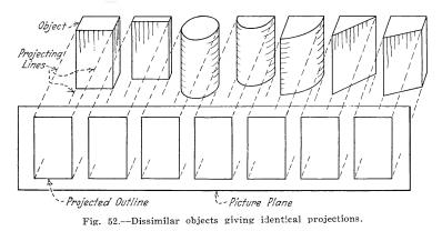
**Orthographic Projection.**—If the observer is considered as having moved an infinite distance away from the plane and the object, the lines of sight (projecting lines) locating the outline will become parallel (Fig. 51b,) and every line parallel to the picture plane will project in its true length.
