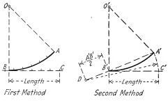
Fig. 84 .- Finding the length of a circular arc.
