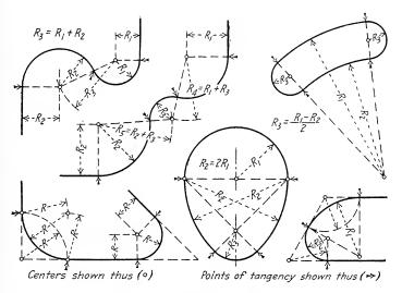
Fig. 86 .-- Construction of tangent arcs.
