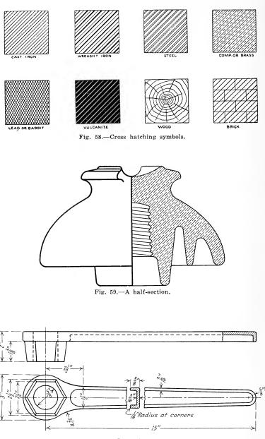
PLUG WRENCH Fig. 60.—A detail drawing.
