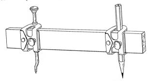
Fig. 25.-A simple form of beam compasses.
