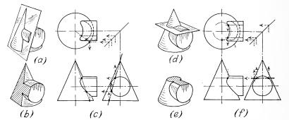
Fig. 64. Two methods of finding points on the line of intersection of a cone and a cylinder.
