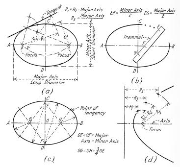
Fig. 87.-Construction of the ellipse and the parabola,
