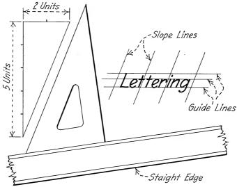
Fig. 35 .- Method of drawing slope lines for lettering.
