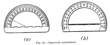
**Protractor.**—While not the most accurate method of measuring and laying out angles, the use of a protractor is one of the most convenient. There are many types available, ranging from the common semi-circular type (Fig. 20) to precise instruments equipped with verniers, micrometer screws, and magnifying glasses for close reading. They are usually made of brass or German-silver, but many excellent styles are now being made of heavy transparent celluloid, it being convenient to en-
