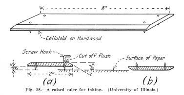
**Raised Ruler**.—Much time can be saved in inking by the use of a short ruler (Fig. 28) supported slightly above the surface of the drawing by four metal points. With this device wet ink lines may be worked over freely and little time need be spent waiting for the ink to dry. The construction is clearly indicated, and any draftsman can well afford to take the time and trouble necessary to make such a ruler.
