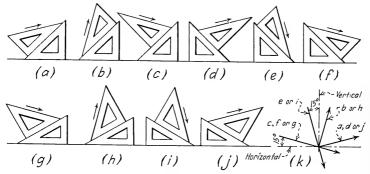
Fig. 6.-The triangles used in combination.
