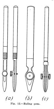
triangle or French curve. The usual pattern is indicated in Fig. 12a, both a front and side view being shown.
