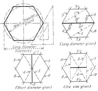
Fig. 85.-Construction of regular hexagons.
