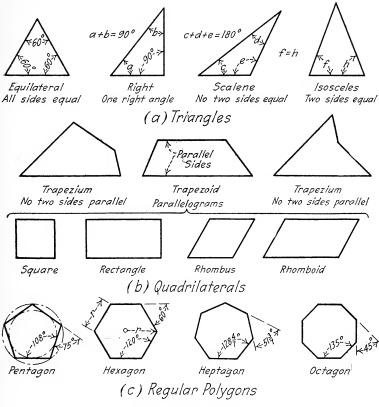
Fig. 80.-Triangles, quadrilaterals and polygons.
