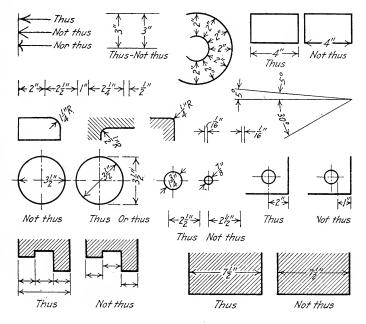
Fig. 68 .- Arrangement of dimensions.
