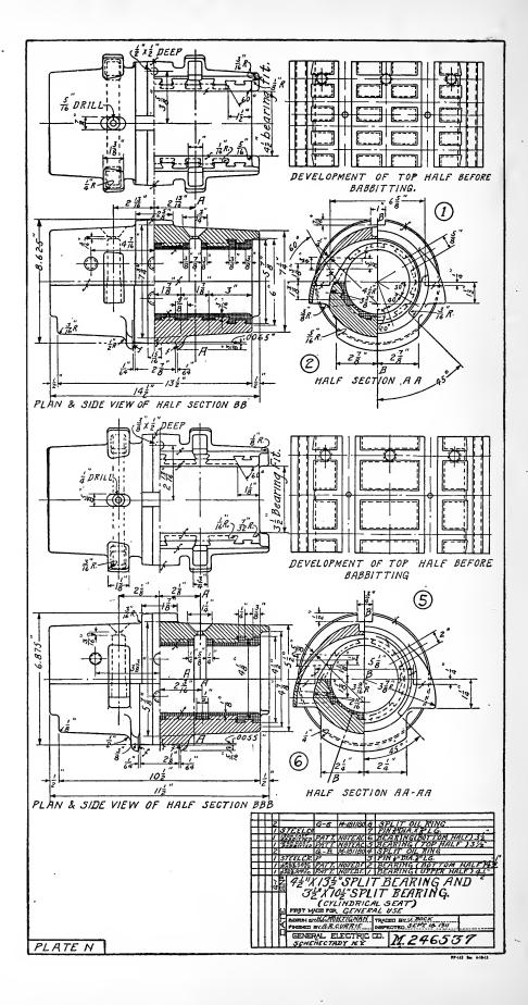
It is necessary, of course, to cut away the metal at this point after it is cold in order to provide a peep hole and in order to clear the slots for the oil rings. The inside surfaces, being shaped to fit after the metal is cold, have grooves for oil transmission cut in after the bearing is complete. Since these operations cannot be shown in the drawing, no information is given except as to the metals being used.
