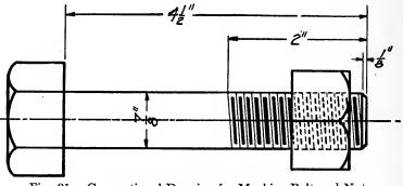
Fig. 21. Conventional Drawing for Machine Bolt and Nut
