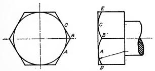
Fig. 23. Conventional Drawing for Machine Bolt Head
