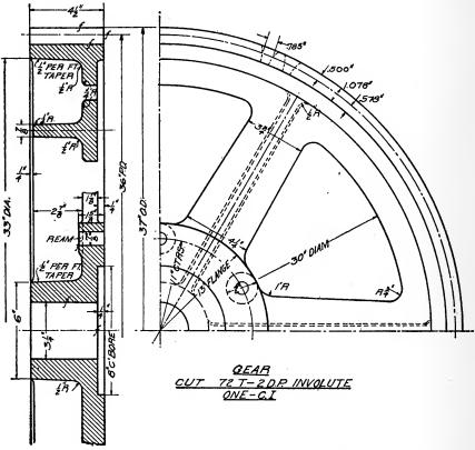
Fig. 40. Detail of Gear with Solid Hub
