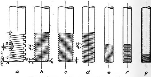
Fig. 17. Conventional Representations of Screw Threads
