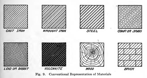
Shade Lines. The theoretical principles for shade lines, already given in Mechanical Drawing, Part III, cannot be exactly applied to working machine drawings without involving an excessive amount of time and labor. The conventional rule, therefore, has been
