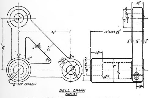
Fig. 33. Method of Showing Dimensions on Detail Drawing
