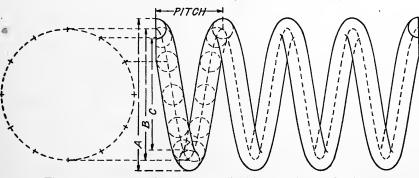
Fig. 56. Accurate Diagram for Helical Spring of Round Wire
