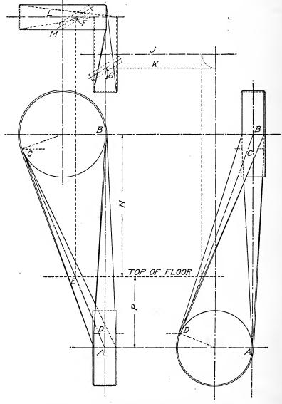
Fig. 110. Locating Belt Holes for Quarter-Twist Drive
