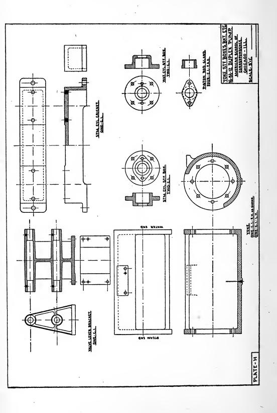
same level as that beneath the water cylinder. The tapped holes in the top surface receive bolts from the cylinder foot. These bolts are often used only for shipping purposes, the cylinder foot when the pump is set up being allowed to slide freely on the cricket, thus permitting free expansion and contraction. In such cases the water end is rigidly fastened to the foundation by holding down bolts.
