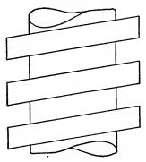
Fig. 75. Conventional Drawing for Square Thread
