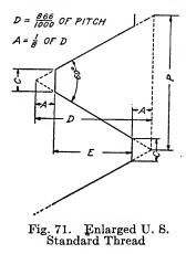
pitch P. The sharp corners, however, are a disadvantage, since on the outside they are likely to be bruised and to give trouble in putting on the nut, and at the bottom of the groove they tend to weaken the bolt or screw. In order to avoid these sharp corners, the threads are flattened in the United States standard thread, as shown in Fig. 71, the amount of this flattening being such that the distance C is  $\frac{1}{8}$  of the pitch, or—what amounts to the same thing—the distance A
