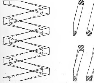
Fig. 59. Conventional Drawing for Square Wire Spring
