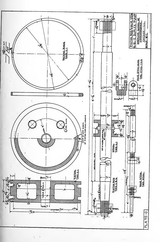
by a nut, and the nut is checked by a  $\frac{1}{4}$ -inch split pin. The packing rings are prevented from slipping round the piston by lugs fitting loosely in chipped recesses in the groove. These being at opposite sides for each groove, the leakage of steam through the split in the ring is minimized, for it must pass halfway around the piston before it can pass through the split in the other ring. This is a simple, but fairly effective, device.
