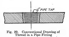
the conventional ways previously explained, but the number of threads per inch and the diameter of the hole need not be given; instead, a note is made that the hole is tapped for a certain size pipe. Fig. 29 illustrates this.
