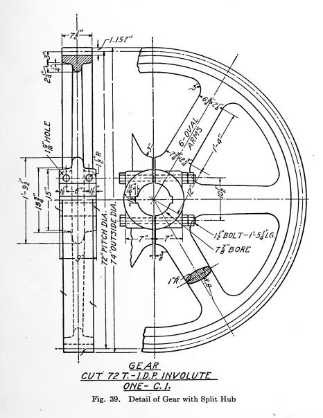
The information which enables the workman to choose the proper cutter is given in the title; thus, "Cut 72 Teeth—1 Diametral Pitch —Involute." The workman will receive from the tool room a standard involute cutter marked for 72 teeth, 1 diametral pitch. After placing same on the arbor of the gear-cutting machine, he will drop the cutter into the gear blank to the depth called for by the drawing;
