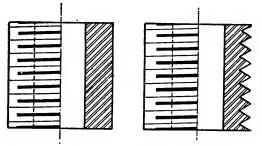
Fig. 20. Conventional Drawing for Threads in Sectional Pieces
