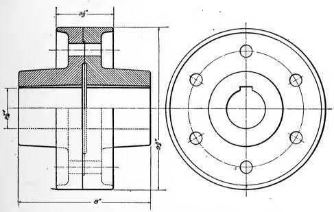
Fig. 2. Flanged Coupling Giving Practical Application of Fig. 1
