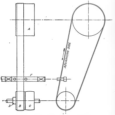
Fig. 96. Diagram of Tight and Loose Pulley Drive
