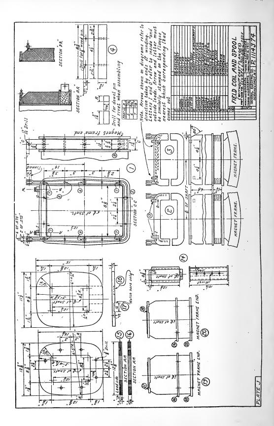
would be called for by number; these numbers in turn being given in the dimension table, would fix the dimensions of the piece wanted. This is a method used in many drafting rooms where many similar pieces are used which can be treated in this way.
