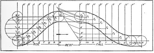
Fig. 91. Diagram Showing Development o fTranslation Cam
