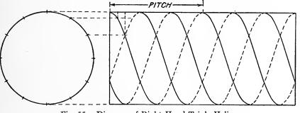
Fig. 55. Diagram of Right-Hand Triple Helix
