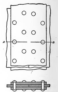
Fig. 8. Butt Joint Showing Use of Crosshatching When Section Is Through Different Pieces of One Material
