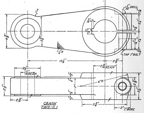
Fig. 32. Detail Drawing of Crank
