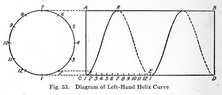
CR is just one-half the pitch. The curve from E to B is the projection of the next turn of the helix and is exactly like the first one.
