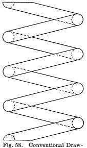
Fig. 58. Conventional Drawing for Spring of Round Wire
