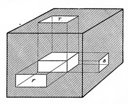
Fig. 3. Rectangular Block Within a Glass Box, the Surfaces Projected to the Top, Front, and Right-Hand Side
