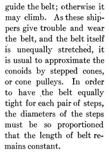
It can be shown, geometrically, that for a crossed belt this condition is obtained when the sum of the diameters of each pair of steps is constant. In Fig. 106, a three-step cone with crossed belt is shown; and, adding together the diameters of the pair of steps connected by the belt, we have 11+6=17 for the constant of this cone pulley.
