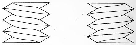
Fig. 61. Simple Drawing for Left and Right-Handed V Screw Threads
