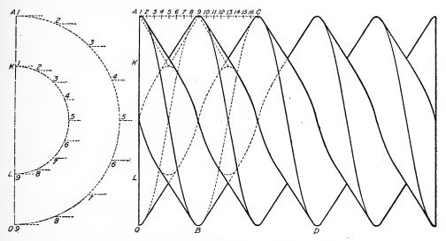
Fig. 63. Accurate Construction for Double V Thread
