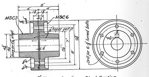
27" Flange Coupling - Steel Casting. 2-Female-MSC 6. Ship with shaft MSI7. 2-Male - MSC 5. Fig. 36. Detail Drawing of a Coupling, Using a Cross-Sectional View
