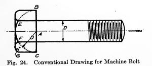
rounded off with a radius equal to about  $1\frac{1}{2}$  times the diameter. The lines which represent the thread should not cross the line drawn square across the bolt where the chamfer or rounding of the point
