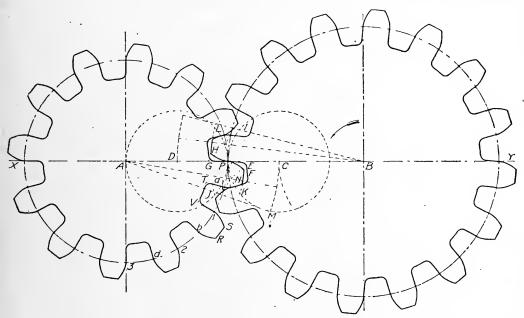
Fig. 114. Construction of Epicycloidal Gears
