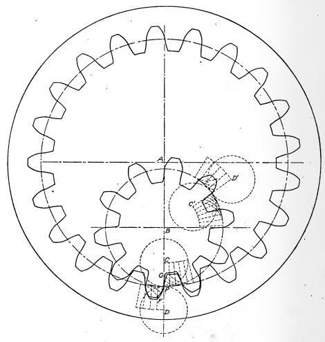
Fig. 115. Layout for Annular Gears
