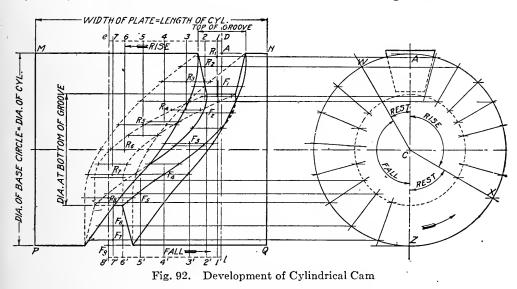
cylinder is rotated on its axis, the cycle of follower movement will be repeated as long as we choose to rotate the cylinder. Such a grooved cylinder is known as a cylindrical cam.
