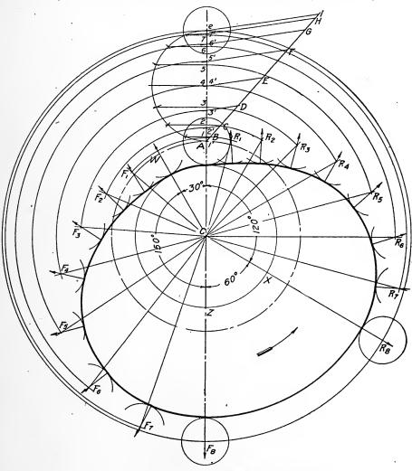
Fig. 90. Diagram of Complex Motion Plate Cam
