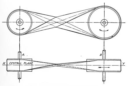
Fig. 94. Diagram of Simple Crossed Belt Drive
