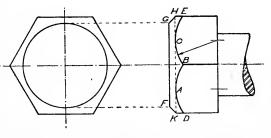
Fig. 26. Hexagonal Bolt Head with Chamfer
