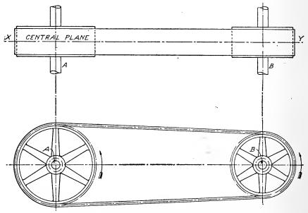
Fig. 93. Diagram of Simple Open Belt Drive
