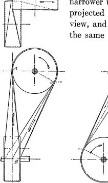
arrangement where two guide-pulleys are used. Let the driving pulley R and the driven pulley P be located as in the case of the quarter-twist belt of Fig. 99. Suppose that the direction of rotation is but seldom reversed, and that the usual motion of the driver is in the direction of the arrow. The part of the belt which has the greater load should have a direct connection between R and P, leaving the slack side to run over the guide-pulleys, thereby decreas-
