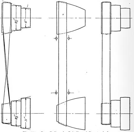
Fig. 106. Cone Pulleys for Spindle and Countershaft
