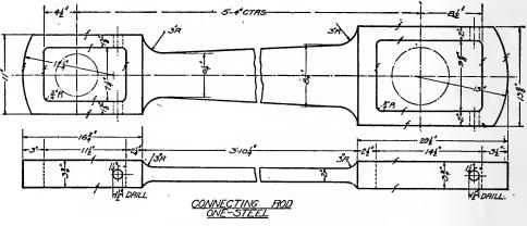
Fig. 38. Detail of a Connecting Rod
