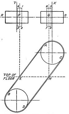
Fig. 108. Diagram Showing Method of Locating Belt Holes
