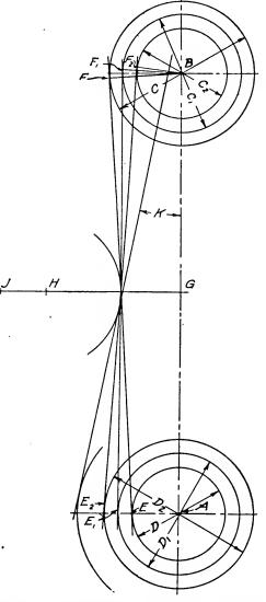
Fig. 107. Diagrammatic Layout for Cone Pulleys
