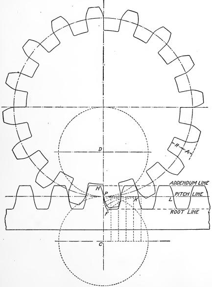
Fig. 116. Construction for Epicycloidal Rack and Pinion
