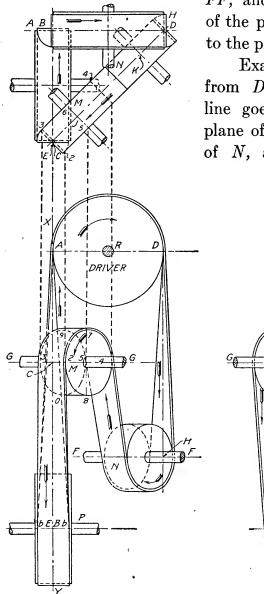
FF, and the corresponding views of the pulleys are drawn according to the principles of projection.
