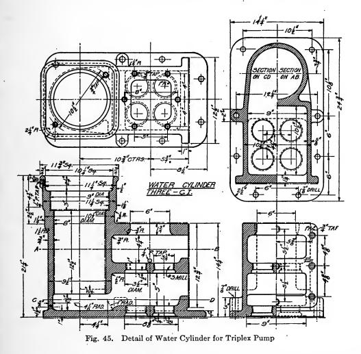
cross-sectional views the dotted lines have been almost entirely eliminated, thereby leaving the section work clear and plain. There is no necessity of showing parts in dotted lines which are beyond the plane of the section, but in several places just enough simple dotted work is shown to convey the relation of the parts.
