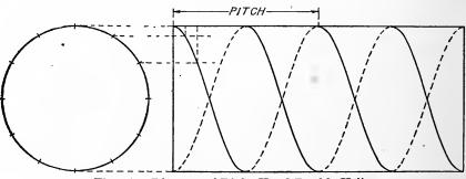
Fig. 54. Diagram of Right-Hand Double Helix
