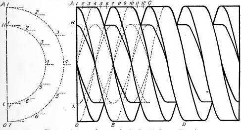
Fig. 66. Accurate Construction for Double Square Thread
