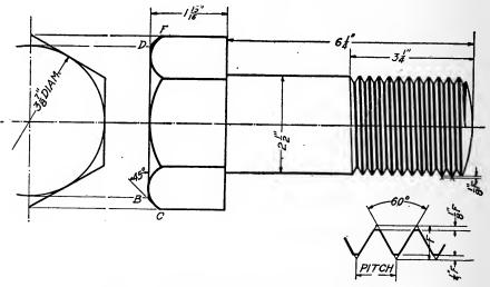
Fig. 25. Machine Bolt with U.S. Standard Thread
