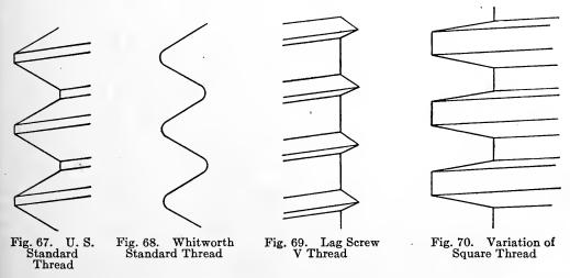
the Sellers or United States standard thread, an enlarged drawing of which is shown in Fig. 71. Referring to this figure, we see that the angle between the two sides of the thread is 60°, so that if the thread came to a point at the top and bottom, as indicated by the dotted lines, the depth of the thread D would be about  $\frac{87}{100}$  of the
