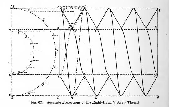
make the drawing are the outside diameter AO, the pitch AC, and the depth of the thread AK. First draw the two projections of a cylinder of a diameter equal to the outside diameter of the screw. Half of the end view is sufficient. On the line AE of this cylinder lay off AC equal to the pitch; starting at A, draw the helix ABCD, as described for Fig. 52. Inside of the cylinder AO, draw a smaller
