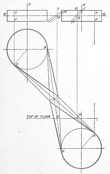
Fig. 109. Diagram Showing Location of Holes for Crossed Belt
