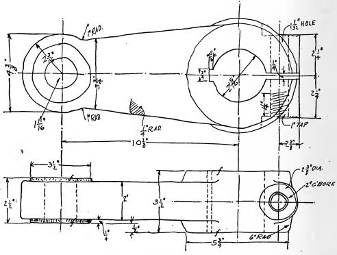
Fig. 31. Preliminary Sketch of Crank
