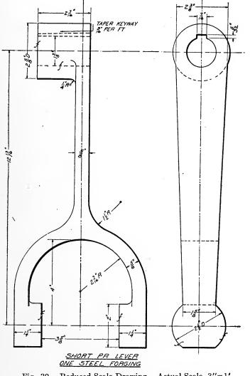
Actual Scale, 3"=1' Fig. 30. Reduced Scale Drawing.
