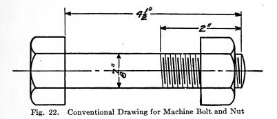
the long diameter is given in preference to the view across the flats, so that in close quarters the clearance of the corners may be readily seen. The shank of the bolt is represented as explained
