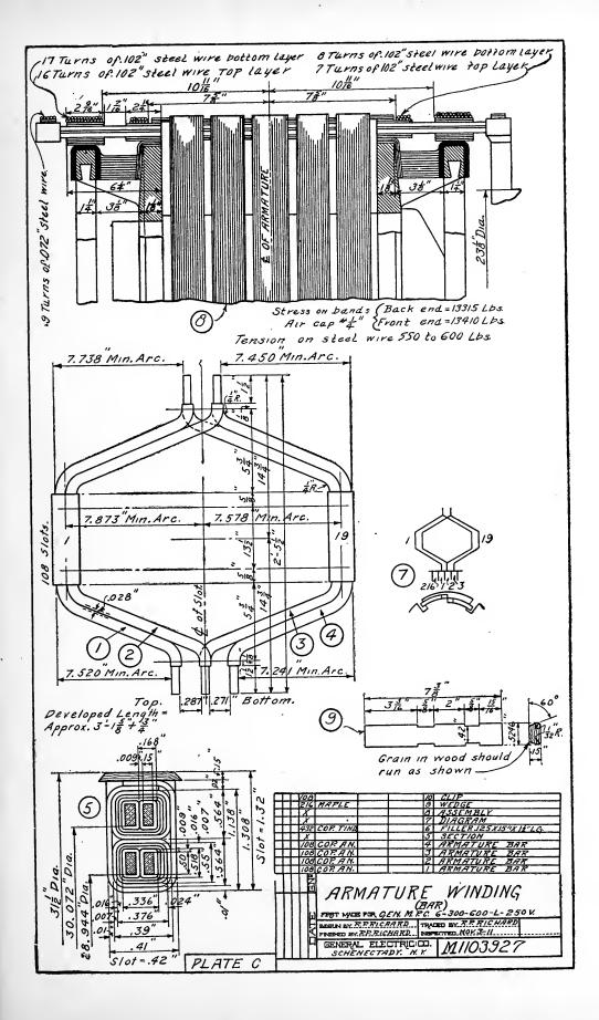
be drawn to a very large scale, such as twice the size, in order that all dimensions may be shown without sacrificing clearness. In this section it should be noted that several diametrical dimensions are given and that the dimensions of the slot are shown along with the corresponding dimensions of the coil.
