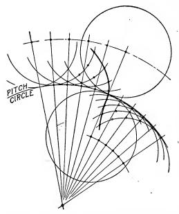
Fig. 113. Methods of Drawing Cycloidal Curves
