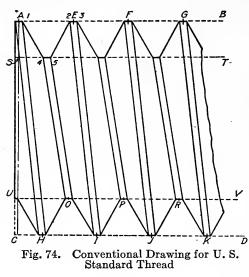
the points thus found, draw lines 1-4, 2-5, etc., making an angle of 60° with AB. The rest of the drawing is completed as shown by drawing in full lines those parts of the lines AB, CD, ST, and UV intercepted between 1-4 and 2-5, etc.
