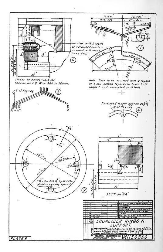
Equalizer Ring Support. From the data already given in Fig. 6 and on Plate D, the support for the equalizer rings may now be drawn, Fig. 7. The principal dimensions are determined from the previous drawings and it only remains to work out the details, which need no explanation.
