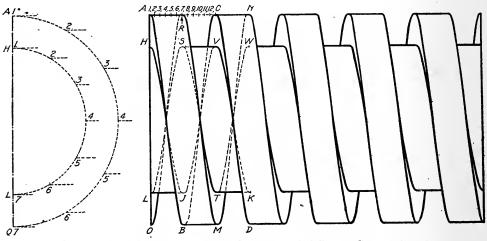
Fig. 65. Accurate Projections for Right-Handed Square Screw Threads
