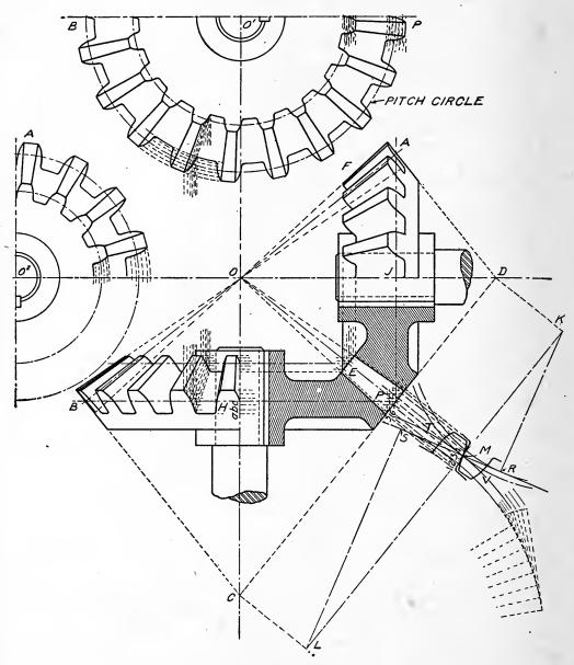
Fig. 119. Construction Diagram for Pair of Bevel Gears
