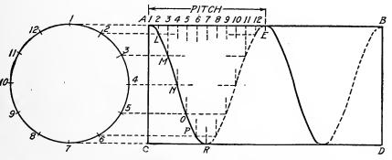
Fig. 52. Diagram Showing Construction of Right-Hand Helix Curve
