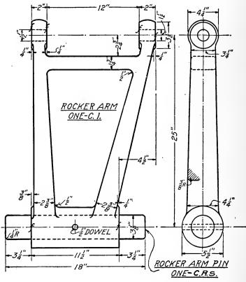
Fig. 34. Detail of Rocker Arm and Pin
