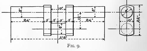
draughtsman, as he is frequently called upon to make sketches from broken pieces of machinery, to be afterwards used as notes from which to make drawings. These sketches consist of outlines giving the form of the object in as many views as may be necessary to show its form and bearing the measurements required for making a correct drawing.
