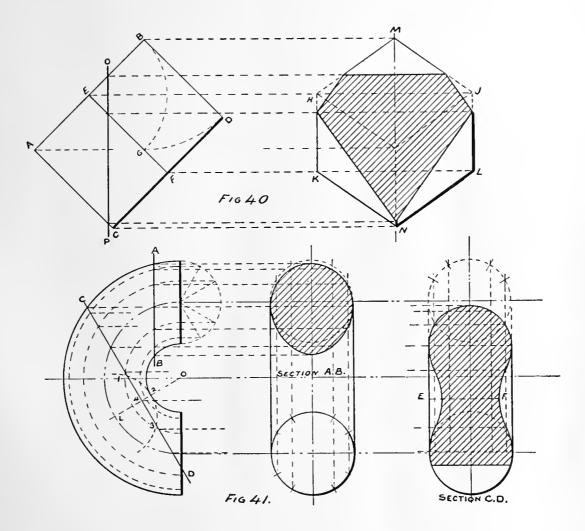
PLATE 37.—A sphere cut by a plane at an angle to its vertical axis. In the side elevation a straight line drawn to the required angle will represent the plane.
