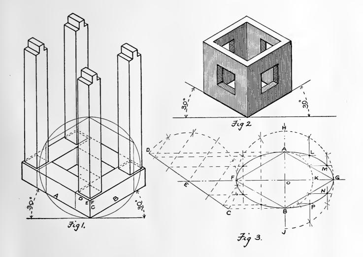
ting A produced in D, draw C D and bisect in E and erect perpendicular. With E for centre and E C for radius draw semi-circle and subdivide, and project the points of subdivision perpendicularly upon D C. With O for centre and radius O G draw semi-circle and subdivide, and proceed as in lesson on Page 52, Plate 7.
