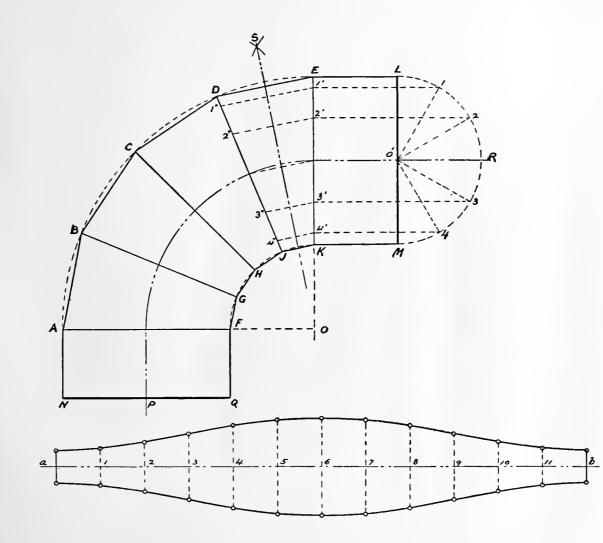
PLATE 32. Intersection of a Small Cylinder with a Large Cylinder at Angle of 30°.
