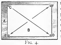
stretch the paper from C to the lower right hand corner D by drawing the palm of the hand in the direction of the arrow, using enough pressure to draw the paper, but not sufficient to tear it away from C, and put in pin D. Next beginning at
