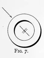
of the light line. To do this, draw first the line representing the cylinder, then find a new centre in a line following the direction of the light, and with the same radius draw another line on the lower right side for the outside, and the upper left for the inside of the cylinder. In Fig. 7 this is shown with
