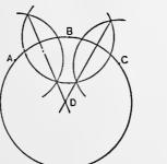
11 To draw a circle through three given points use the same construction as used for No. 10, the centre D being found by the same method.
