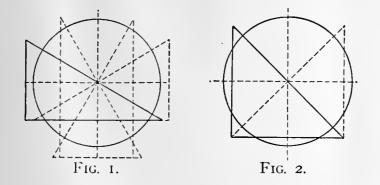
Hold triangle A firmly with the left hand and slide triangle B along in either direction, holding it firmly against A, to the point through which the line is to be drawn.
