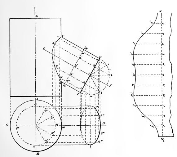
PLATE 33. To Lay Out the Envelope of a Cone.
