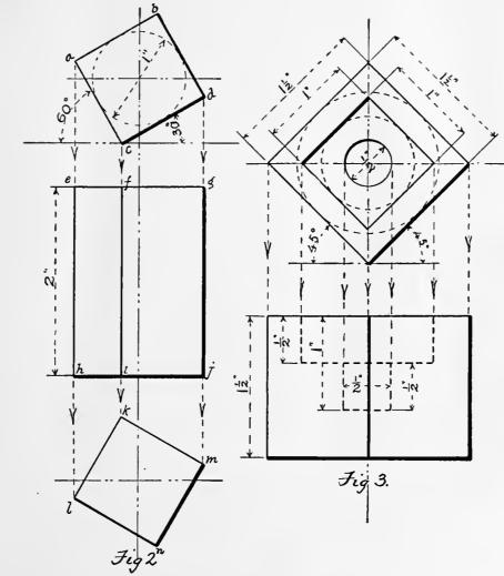
FIG. 3.—A cube resting upon one of its edges with sides at angles of 45° to horizontal. In one face of the cube is a depression 1″ square,  $\frac{1}{2}$ ″ deep, while in the centre of this depression is a further depression, round  $\frac{1}{2}$ ″ diameter,  $\frac{1}{2}$ ″ deep, the cube being  $1\frac{1}{2}$ ″ square on each face.
