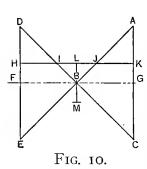
so that their apexes join, and if their axes, B G, B F, are in the same straight line, and they are cut by the same plane, H I L J K, parallel with F B G, the sections thus obtained will form two hyperbolas, N J O and P I Q, as shown in Fig. 11, which are called the *branches* of the hyperbola. I and J are the *ver*-
