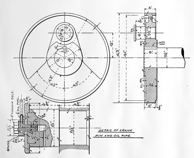
DISC CRANK AND CRANK PIN.
