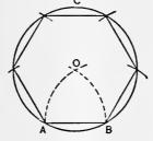
radius step off points around the circumference; connect these points to complete the hexagon.
