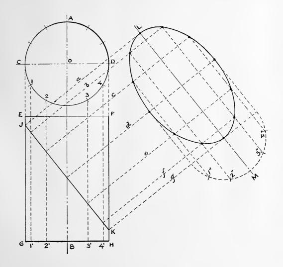
PLATE 13.—To draw an ellipse when the long and short diameters are given:
