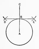
14. To draw tangents to a circle from a point without the circle. Let E be the given point. Join D and E and on D E as a diameter draw the circumference intersecting the
