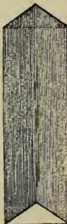
$$\begin{aligned} \sqrt{2.5^2 + 2.5 \times 2.5} &= 2.165+ = \text{sine of angle, or depth of base ; or,} \\ 2.5 \times 3 \times .28868^* &= 2.165+ = \text{height of triangle ; and} \\ 2.165 \times 2.5 &= 2.706+ = \text{area of base ; or,} \\ 2.5^2 \times .433012^* &= 2.706325 = \text{area of base ; and} \\ 2.706+ \times 12 &= 32.475+ \text{ cubic feet. } \textit{Ans.} \end{aligned}$$
