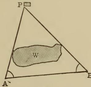
tance from a point  $A$  to an inaccessible object  $P$ ; further, imagine a wood  $W$  so situated that  $B$  would be the first point to the right of  $A$  from which an unobstructed view of  $P$  could be obtained. Now, we might lay off a known length  $AB$  (called a base line) and with a transit, measure the angles  $BAP$  and  $ABP$ ; we could then calculate the
