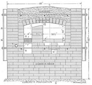
Fig. 8. Case-hardening Furnace. Section in A-B, Fig. 9
