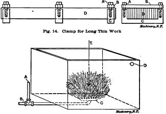
Fig. 15. Hardening Tank Arranged for Mottling and Coloring
