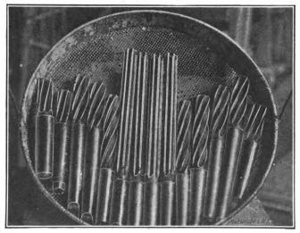
Fig. 16. Hardened Reamers, just Removed from Oil Bath
