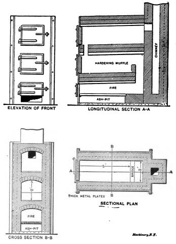
Fig. 6. Plan and Elevation of Flather Case-hardening Furnace
