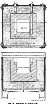
ig. 5. Section of Electrical Hardening Furnace
