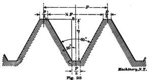
In the illustration, p is the pitch of the thread. The pitch, of course, equals  $\frac{1}{1}$ .\* It is required to find the depth BC No. of threads per inch.
