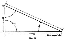
As a further example, assume that the sides forming the right angle are given as shown in Fig. 21; one is 15 inches and the other is 36 inches. Find the hypotenuse and the angles B and C.
