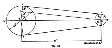
Now, AK is the radius of the larger pulley, which is one-half its diameter, or 6 inches, and HC is the radius of the smaller pulley or 3 inches. Hence, GK = 6 - 3 = 3 inches. HK = 5 feet or 60 inches, as given in the problem. We then have here a right-angled triangle in which the hypotenuse HK = 60 inches, and one of the sides forming the right angle is 3 inches. Hence, side GH is found by the formula given for this case in the previous chapter, and by inserting the known values we have:
