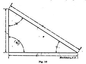
A is the right angle in the triangle. The side a opposite the right angle is the hypotenuse. The side b is called the side adjacent to the angle C, but is of course also the side opposite to angle B. In the same way, the side c is called the side adjacent to angle B, and the side opposite to angle C. The reason for these names is made clear by studying the figure.
