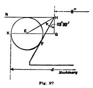
*Example* 5.—Small reamers are sometimes provided with flats instead of actual flutes. The diameter of the reamer is, of course, measured over the sharp corners; if the reamer tapers, the taper of the flats will not be the same as the taper of the sharp corners, and the milling machine dividing head must be set to a different angle from that which the cutting edge makes with the center line. A simple formula may be deduced by the
