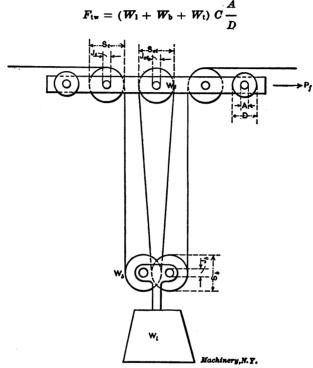
Fig. 14. Trolley with Sheave Suspended by Four Parts of Rope
