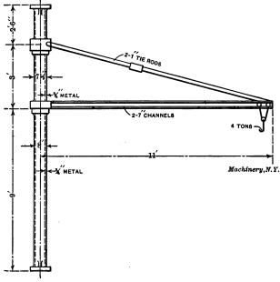
Fig. 5. General Construction of Jib Crane in Problem 1
