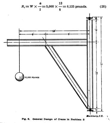
This produces a tensile stress in DH which may be found by the parallelogram of forces shown in Fig. 9, or by the following calculation:
