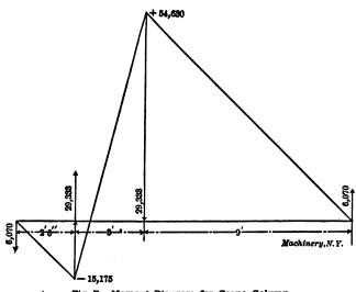
Fig. 7. Moment Diagram for Crane Column
