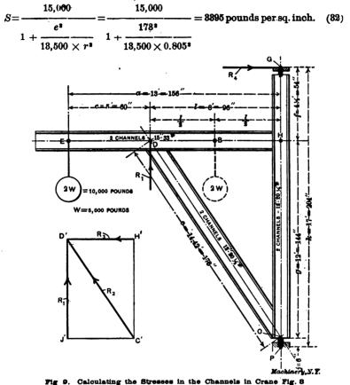
The reaction producing compression in CD is found by the force diagram in Fig. 9, or by the following calculation:
