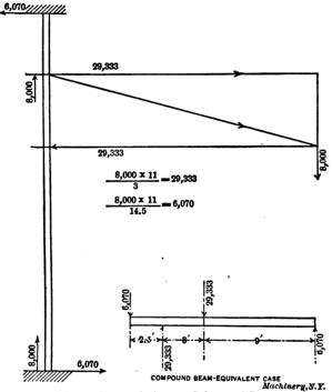
Fig. 6. Forces Acting on Column of Crane
