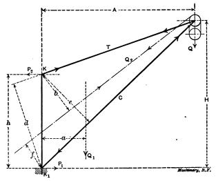
Fig. 17. Diagrammatical View of Pillar Crane
