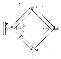
Fig. 35. Double Toggle-Joint.
