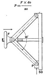
Fig. S4. Toggle-Joint Design where Pressure is Exerted by Handwheel and Screw.
