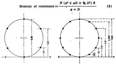
Figs. 14 and 15. Finding the Stress on the Bolts for Six and Twelve Bolts. When the neutral axis lies inside of the bolt circle we have  $(0-\phi) + (a-\phi) + (b-\phi) + (c-\phi) + \ldots$  which may be written  $N\phi^2 - 2\phi (a+b+c+\ldots) + a^2 + b^2 + c^2 + \ldots$  and for the moment we have
