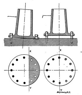
Figs. 10 and 11. Location of Neutral Axis under Varying Conditions.
