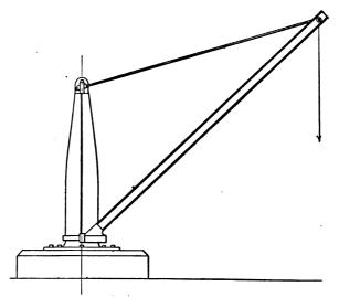
Fig. 7. Jib Crane; Load has a Tendency to Overturn.
