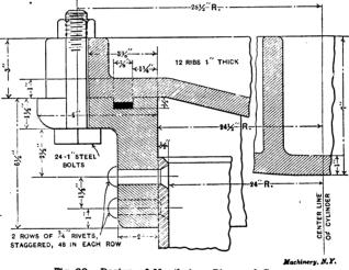
Fig. 20. Design of Mouthpiece Bing and Cover.
