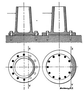
Figs. 12 and 13. Location of Neutral Axis under Varying Conditions.
