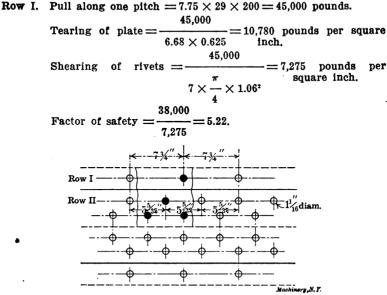
Fig. 18. Joint Re-designed to give Less Stress in Row II than in Row I.
