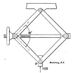
Fig. 86. Alternative Design of Double Toggle-Joint.
