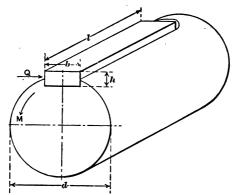
Fig. 25. Shaft with Ordinary Rectangular Key.
