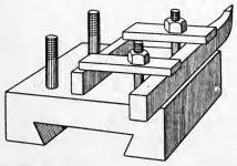
Fig. 119. Tool Holder for Heavy Turning
