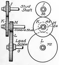
Fig. 98. Compounding Gears
