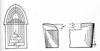
Fig. 368. Taylor Standard Cutting Contours Courtesy of Ready Tool Company, Bridgeport, Connecticut
