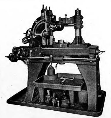
Fig. 283. Automatic Gear-Cutting Machine Courtesy of D. E. Whiton Machine Company, New London, Connecticut
