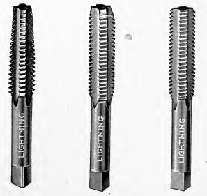
Fig. 81. Types of Hand Taps: Left—Taper Tap; Center—Plug Tap; Right—Bottoming Tap Courtesy of Wiley and Russell Manufacturing Company, Greenfield, Massachusetts
