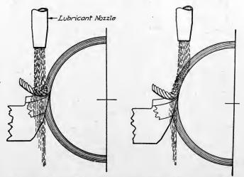
Fig. 373. Right and Wrong Method of Feeding Lubricant to Cutting Tool Courtesy of "Machinery", New York City
