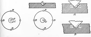
Fig. 178. Layout for Drilling Hole
