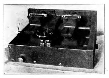
Fig. 390. Typical Milling Fixture
