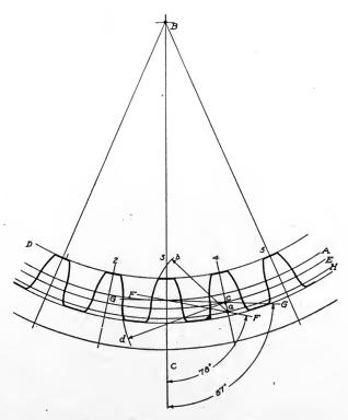
Fig. 267. Laying Out Teeth of Internal Gear
