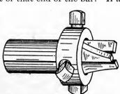
Fig. 323. Improved Hollow Mill
