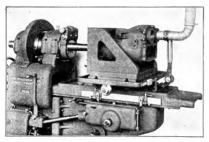
Fig. 334. Grinding Gas Engine Cylinders. View Shows Exhaust for Dust, Jig for Holding Cylinders, and Eccentric Wheel Spindle Courtesy of Heald Machine Company, Worcester, Massachusetts
