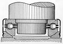
Fig. 394. Hess-Bright Thrust Bearing with a Lining Washer and Enclosing Case
