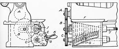
Fig. 99. End and Front Elevation of Rapid Change-Gear Device
