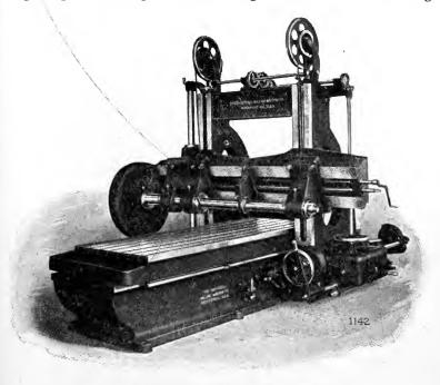
Fig. 225. Slabbing Miller—Planer Type Courtesy of Ingersoll Milling Machine Company, Rockford, Illinois
