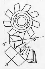
Fig. 244. Cutting a Bevel Gear
