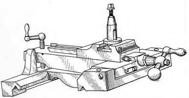
Fig. 122. Tool-Post with Rise-and-Fall Rest
