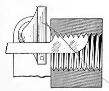
Fig. 168. Hand Chaser Cutting Inside Thread
