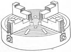
Fig. 104. Lathe Work Chuck
