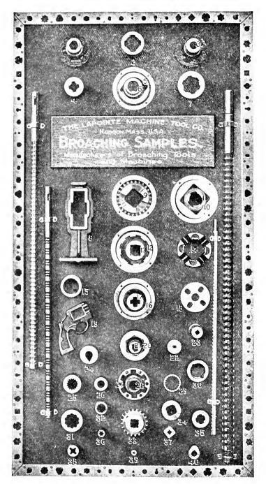
Fig. 367. Samples of Broaching Work Courtesy of LaPointe Machine Tool Company, Hudson, Massachusetts
