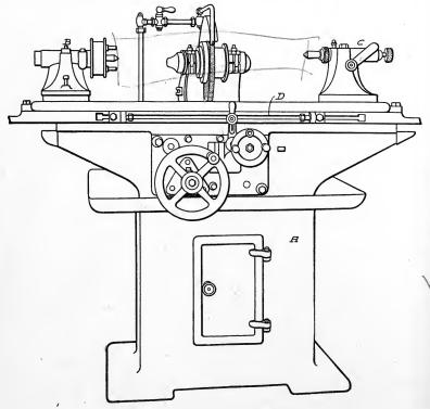
Fig. 247. Cylindrical-Grinding Machine
