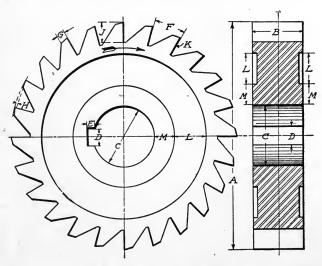
Fig. 200. Details of Ordinary Milling Cutter
