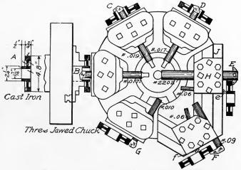
Fig. 310. Arrangement for Machining Spur-Gear Blank
