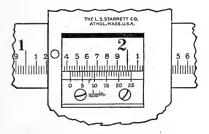
Fig. 25. Enlarged View of Vernier
