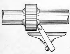
Fig. 93. Hand-Turning a Fillet
