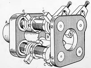
Fig. 307. Box Tool Holder for Two Tools and Four Back-Rest Jaws
