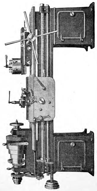
Fig. 294. Engine Lathe with Hand-Revolved Turret Mounted on Latterally Moving Slide
