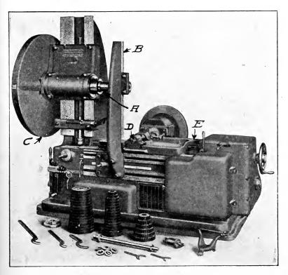
Fig. 284. Number 6 Gear-Cutting Machine Courtesy of Brown and Sharpe Manufacturing Company, Providence, Rhode Island
