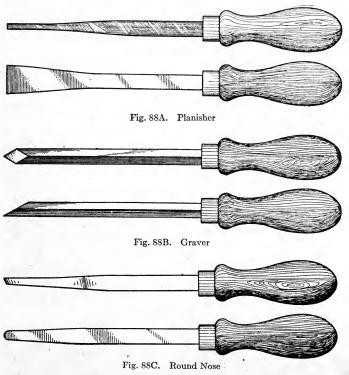
Fig. 88. Cutting Tools for Hand Turning
