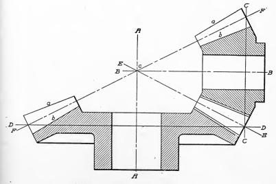
Fig. 271. Cross-Section of Pair of Bevel Gears
