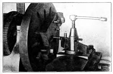
Fig. 388. Boring Hole for Guide Bushing
