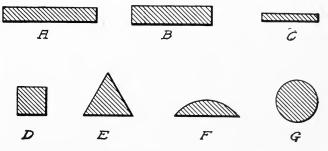
Fig. 49. Cross-Section of Files
