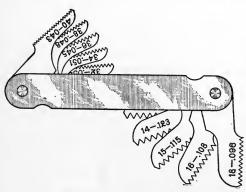
Fig. 163. Screw Pitch Gage
