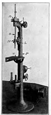
Fig. 174. Sensitive Driller Courtesy of Washburn Shops, Worcester, Massachusetts
