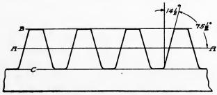
Fig. 268. First Method of Laying Out Teeth of Rack
