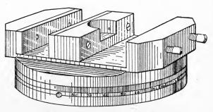
Fig. 189. Planer Chuck for Holding Work
