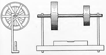
Fig. 257. Method of Using Level for Lining Shafting
