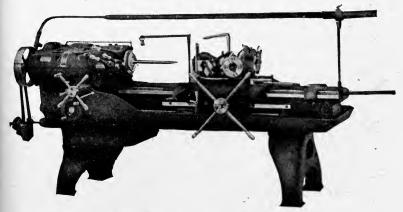
Fig. 299. Flat Turret Lathe, with Special Tools Bolted to Top of Flat Plate Courtesy of Jones and Lamson, Springfield, Vermont
