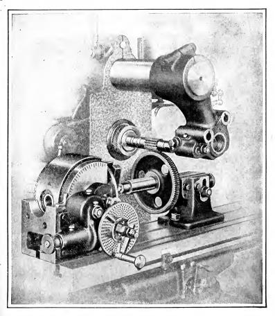
Fig. 245. Hobbing Teeth in Worm Wheel Courtesy of Brown and Sharpe Manufacturing Company, Providence, Rhode Island
