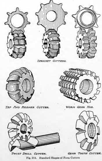
ters for fluting taps, reamers, and twist drills; cutters for sprocket and gear teeth; and cutters known as hobs, for the production of worm gears, Fig. 214. End Mills. All the cutters thus far mentioned are provided with central holes, and are intended to be mounted on an arbor
