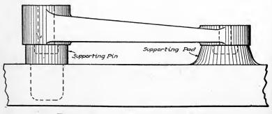
Fig. 381. Sketch Showing Adjustable Locating Points
