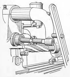
Fig. 238. Milling Spirals with Table at Angle
