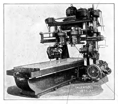
Fig. 226. Planer Type Four-Spindle Milling Machine Courtesy of Ingersoll Milling Machine Company, Rockford, Illinois
