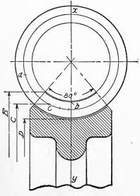
Fig. 273. Worm Gear with Large Enclosing Angle
