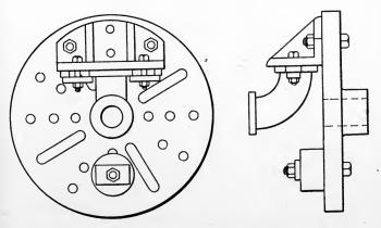
Fig. 137. Angle Iron Clamped to Faceplate and Counterbalanced
