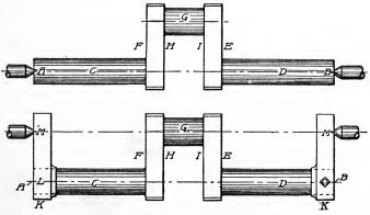
Fig. 148. Machining Crank Shaft
