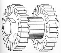
Fig. 207. Side Milling Cutters Mounted as a Heading or Straddle Mill
