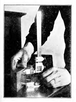
Fig. 387. Positioning Buttons with Vernier Caliper
