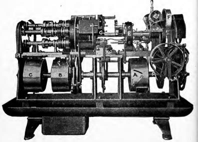
Fig. 317. Universal Multiple-Spindle Automatic Screw Machine
