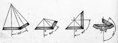
Fig. 270. Bevel Gears at Various Angles
