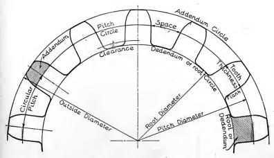
Fig. 201. Names of Tooth Parts
