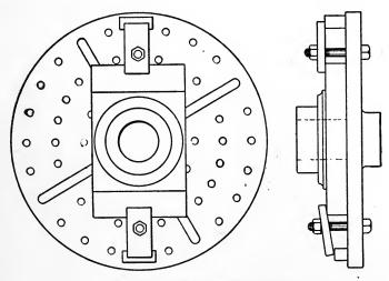
Fig. 135. Work Clamped to Faceplate
