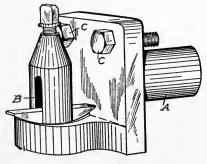
Fig. 306. Turret Holder for Tool-Post
