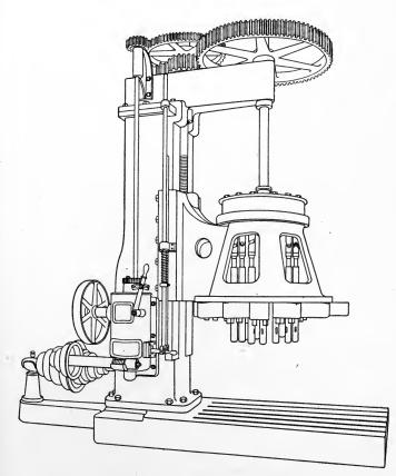
Fig. 176. Typical Multi-Spindle Driller
