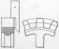
The gear blank is usually mounted upon an arbor fitting in a taper-reamed hole in the index spindle, and
