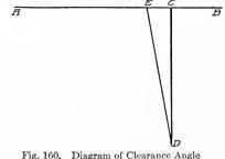
of the side of the cutting tool must be a little greater for clearance. Cutting Tool for Inside Threads. For cutting inside threads, the shape of the cutting edge of the tool should be the same as for cutting an outside thread, and the tool must be made so that the cutting edge alone touches the work. This is accomplished by bending the tool as shown in Fig. 161, and giving it considerable clearance.
