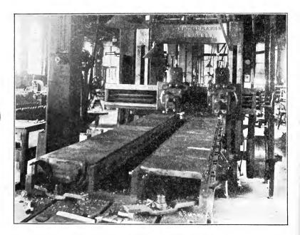
Fig. 392. Typical Planer Fixture, Showing Set-Up for Planing Twenty Square Tables at One Setting Courtesy of Worcester Polytechnic Institute Shops, Worcester, Massachusetts
