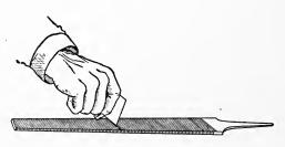
Fig. 55. Removing Pins from a File
