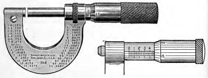
Fig. 21. Ordinary Micrometer Caliper Showing Typical Reading
