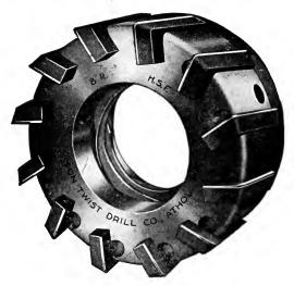
Fig. 345. High-Power Face Mill with High-Speed Steel Teeth Courtesy of Union Twist Drill Company, Athol, Massachusetts
