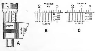
Fig. 23. Diagrams Showing How to Read Micrometer Caliper
