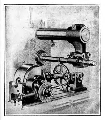
Fig. 242. Cutting Spur Gear on Milling Machine Courtesy of Brown and Sharpe Manufacturing Company, Providence, Rhode Island
