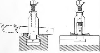
Fig. 118. Tool-Post Holding Tool to Carriage
