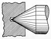
Fig. 133. Hole and Center of Correct Angle for Centering Work
