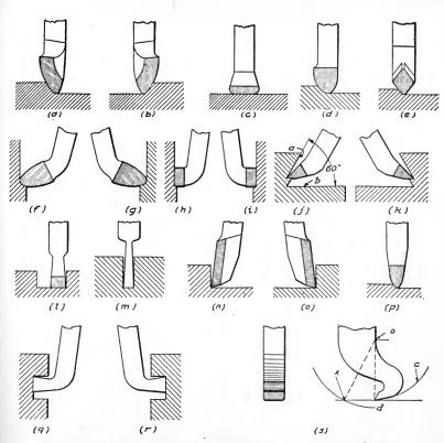
Fig. 372. Planer Tools of Different Form and Work to Which They Are Adapted Courtesy of "Machinery", New York City
