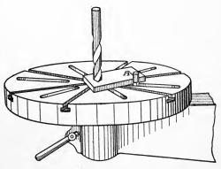
Fig. 182. Use of Table Stud for Drilling
