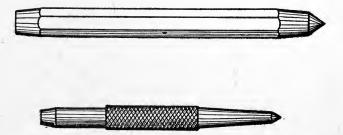
Fig. 60. Hand Punches. Forged Center Punch Above; Prickpunch Below
