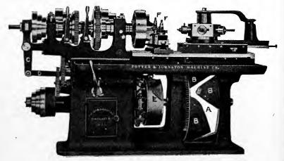
Fig. 313. Automatic Chucking and Turning Machine Courtesy of Potter and Johnston Machine Company, Pawtucket, Rhode Island
