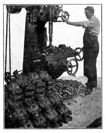
Fig. 348. Baker Driller Driving 22-Inch Drill through Drop-Forged Wrought-Iron Saddles Courtesy of Baker Brothers, Toledo, Ohio
