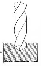
Fig. 70. Drill with Lips of Unequal Angles
