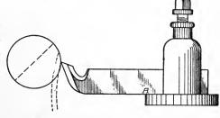
Fig. 185. Lathe Tool Improperly Set Up
