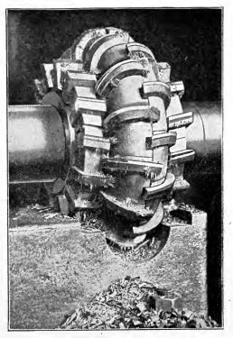
Fig. 346. Production Milling Cutter in Heavy Work Courtesy of Ingersoll Milling Machine Company, Rockford, Illinois
