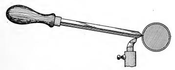
Fig. 92. Position of Tool for Turning Steel
