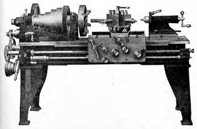
Fig. 293. Engine Lathe with Hand-Revolved Turret on Carriage in Place of Tool-Block
