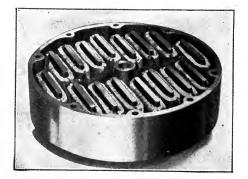
Fig. 400. View of Magnetic Chuck Casting and Unit Coils Courtesy of Heald Machine Company, Worcester, Massachusetts
