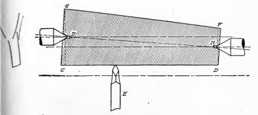
Fig. 144. Turning a Taper by Setting over Dead Center
