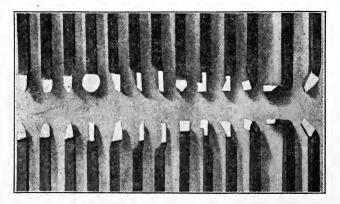
Fig. 371. Set of Planer Tools Ground on Sellers' Tool-Grinding Machine Courtesy of "Machinery", New York City
