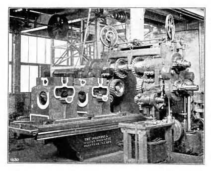
Fig. 343. Ingersoll Horizontal Milling Machine, Milling Gasoline Traction Enzine Frames. <sup>1</sup>/<sub>2</sub> Inch of Metal Removed from each of Six Surfaces. 14 Bases Finished in 10 Hours.
