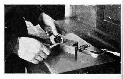
Fig. 386. Positioning Buttons with Micrometer Caliper
