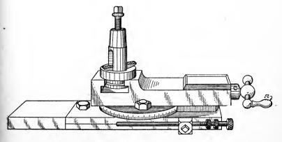
Fig. 146. Compound Tool Slide
