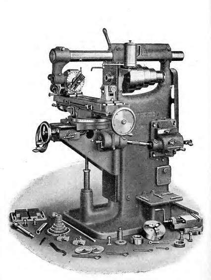
HEAVY UNIVERSAL MILLING MACHINE Courtesy of Brown and Sharpe Manufacturing Company, Providence, Rhode Island
