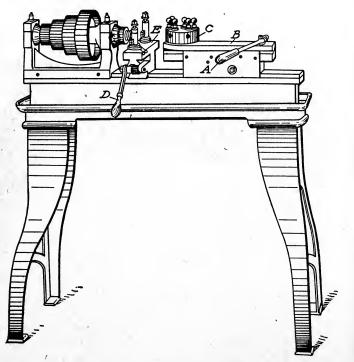
Fig. 292. Form of Monitor Lathe
