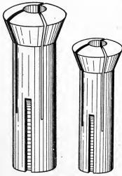
Fig. 221. Typical Spring Collets
