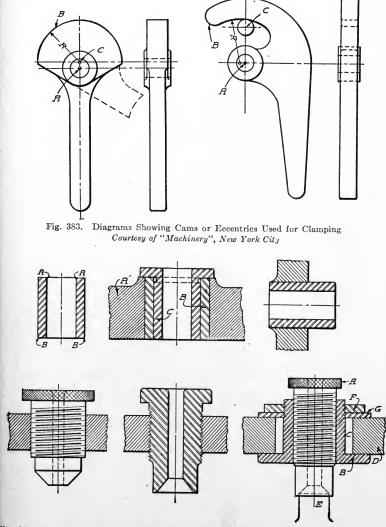
Fig. 384. Typical Bushings: Upper Line—Guiding Lining Bushings for Drill Jigs; Lower Left—Screw Bushing for Locating Work Central with Hole; Lower Center—Screw Bushing for Locating Round Work by Recesses; Lower Right—Floating Bushing Courtesy of "Machinery", New York City
