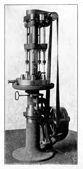
Fig. 350. "Single Purpose" Bemis Driller
