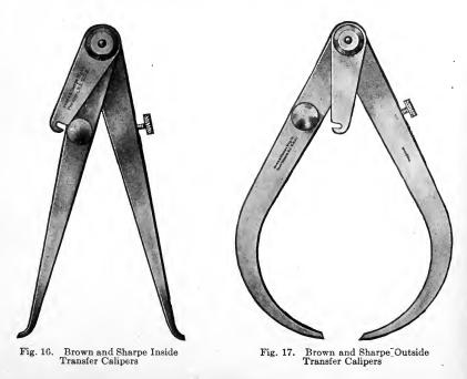
the size of calipers is also designated by the distance from the joint to the end of the leg. Spring calipers are made in sizes from  $2\frac{1}{2}$  to 8 inches, while the other styles vary up to 24 inches.
