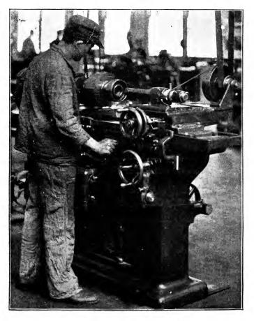
Fig. 398. Heald Internal Grinder Fitted with Magnetic Chuck Courtesy of Heald Machine Company, Worcester, Massachusetts
