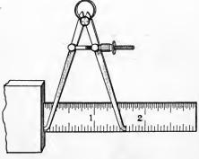
Fig. 18. Setting Inside Calipers
