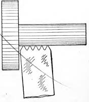
Fig. 167. Hand Chaser Cutting Outside Thread
