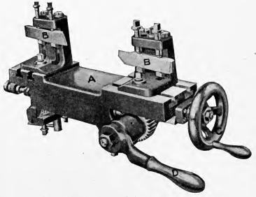
Fig. 308. Cross-Slide Carrying Two Tools
