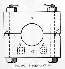
filling pieces CC. The piece is firmly bolted to the faceplate by the bolts DD. The lathe is then run at high speed, and the interior bored out exactly the size of the piece that is to be held. The nuts of the bolts EE are slackened, and the filling pieces CC removed. The piece to be worked on is then inserted, and by tightening the nuts EE, it is securely clamped between the pieces A and B.
