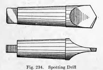
which require accurate placing. The graduated feeds of the milling machine allow the distances to be set off as closely as .00025 inch, and holes can also be drilled to a given depth with equal accuracy. In starting holes, it is best to use a spotting drill, Fig. 234, which is extremely rigid and per-
