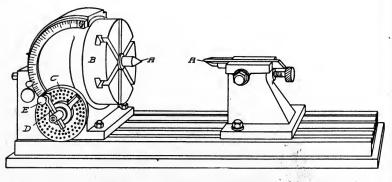
Fig. 243. Gear Cutter with Divided Head
