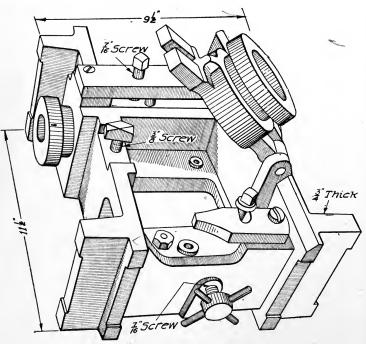
Fig. 377. Two Views of Closed Box Drill Jig Courtesy of "American Machinist"
