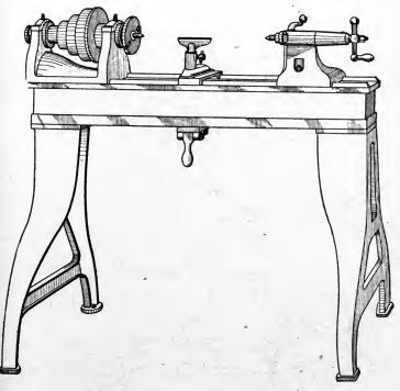
Fig. 87. Typical Speed Lathe for Hand Turning
