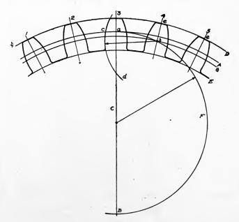
Fig. 264. Laying Out Large Gears
