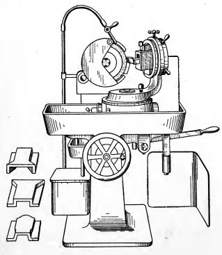
Fig. 132. Tool-Grinding Machine
