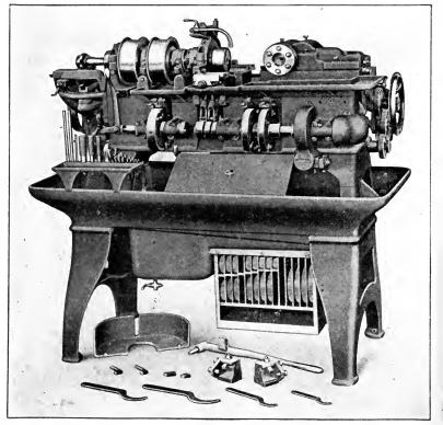
Fig. 321. Number 2 Automatic Screw Machine Courtesy of Brown and Sharpe Manufacturing Company, Providence, Rhode Island
