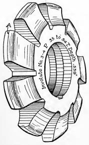
Fig. 279. Rotating Cutter for Involute Teeth
