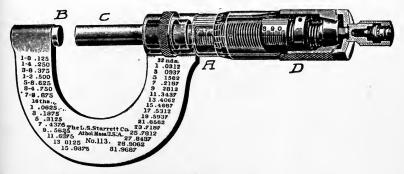
Fig. 20. Transparent View of Micrometer Caliper with Friction Stop Courtesy of L. S. Starrett Company, Athol, Massachusetts
