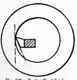
Fig. 129. Boring Tool Set for Clearance tool is shown in Fig. 128. The length of the shank depends on the depth of the hole to be bored, for it must be long enough to reach from the tool-post to the bottom of the hole. This overhang makes the tool more likely to spring, and necessitates a much lighter cut being taken than when removing the same amount of metal by outside turning tools. The result of this lighter cut is seen in the increase of time
