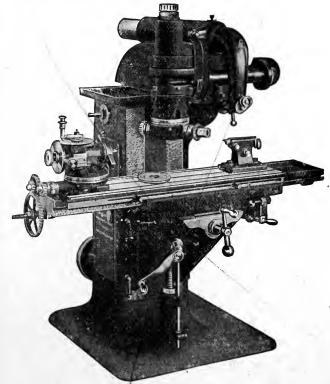
Fig. 231. Duplex Milling Machine Set for Cutting Spirals Courtesy of Van Norman Machine Tool Company, Springfield, Massachusetts
