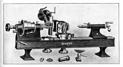
Fig. 222. Rivett Lathe with Milling Attachment Courtesy of Rivett Lathe Manufacturing Company, Boston, Massachusetts
