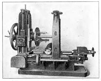
Fig. 285. "New Type" Gear-Cutting Machine Entirely Automatic for Cutting Spur Gears Only Courtesy of Gould and Eberhardt, Newark, New Jersey
