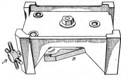
Fig. 375. Typical Open Box Drill Jig Courtesy of "American Machinist"
