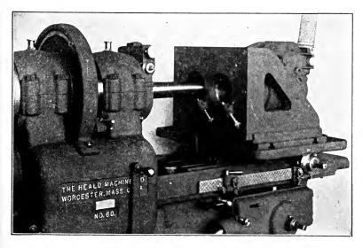
Fig. 335. Grinding Gas Engine Cylinders. Same Set-Up as Fig. 331, Showing Holding Jig and Turning Tool at Mouth of Hole
