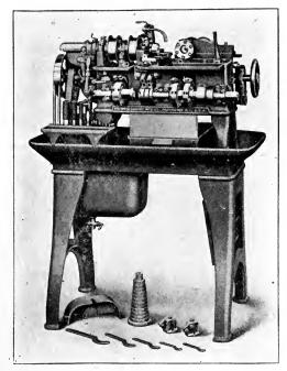
Fig. 318. Brown and Sharpe Automatic Screw Machine, No. 00 Size Courtesy of Brown and Sharpe Manufacturing Company, Providence, Rhode Island
