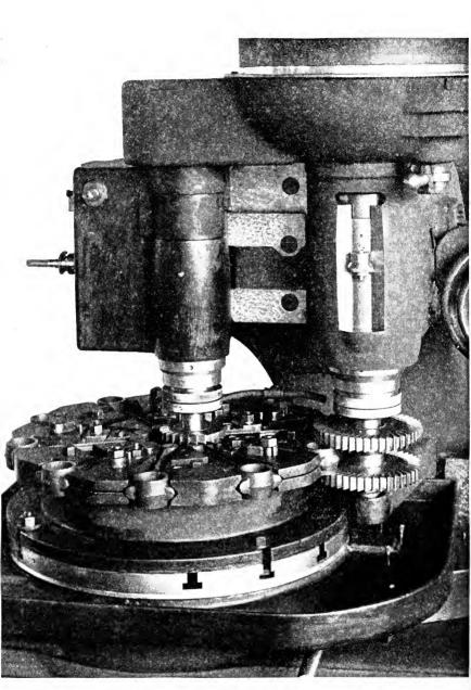
VIEW OF EECKER CONTINUOUS MILLER MILLING CONNECTING-ROD FIXTURE Courtesy of Becker Milling Machine Company, Hyde Park, Massachusetts
