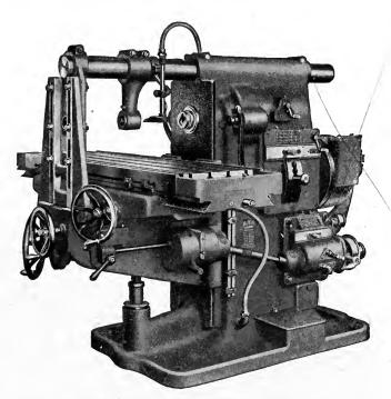
Fig. 224. Horizontal Milling Machine-Column Type Courtesy of Brown and Sharpe Manufacturing Company, Providence, Rhode 1 sland
