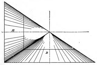
Fig. 259. Two Cones in Contact
