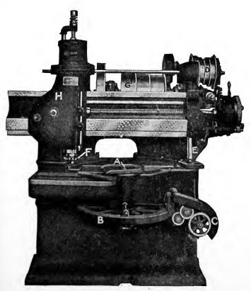
Fig. 288. Gear Shaper Courtesy of Fellows Gear Shaper Company, Springfield, Vermont
