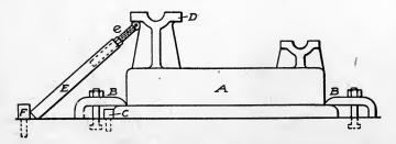
Fig. 187. Method of Clamping Down Planing Machine Bed and Supporting Work
