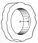
Fig. 138. Centering a Hollow Piece
