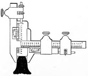
Fig. 280. Gear-Tooth Caliper in Use
