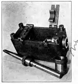
Fig. 391. Typical Boring Fixture
