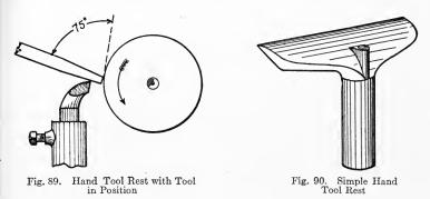
end of a piece of work. The graver can be used on brass for a great variety of operations; but its use, except in the hands of an expert workman, is attended by the danger of catching in the soft metal and thus breaking the tool or spoiling the work.
