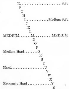
The intermediate letters between those designated as soft, medium soft, etc., indicate so many degrees harder or softer; e.g., L is one grade or degrees softer than medium; O, two degrees harder than medium, but not quite medium hard.
