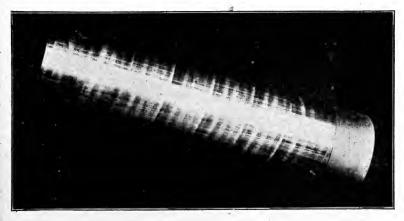
Fig. 326. Traverse Markings on Piece of Ground Work
