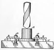
Fig. 181. Work Clamped to Table by Straps for Accurate Hole-Drilling
