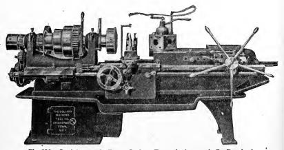
Fig. 296. Semi-Automatic Turret Lathe. Turret is Automatically Revolved at End of Each Stroke Courtesy of Bullard Machine Tool Company, Bridgeport, Connecticut
