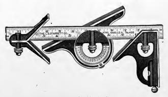
Fig. 11. Combination Set Courtesy of L. S. Starrett Company, Athol, Massachusetts
