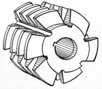
Fig. 278. Hob for Forming Teeth of Worm Gears
