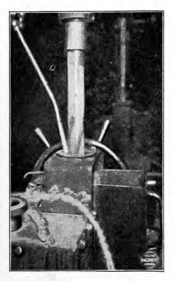
Fig. 374. Drilling Operation Showing How Lubricant Floods the Work Courtesy of "Machinery", New York City
