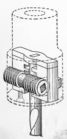
Fig. 169. Drill Held by Drill Chuck
