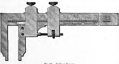
Fig 19. Caliper Square Courtesy of Brown and Sharpe Manufacturing Company, Providence, Rhode Island
