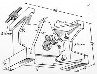
Fig. 376. Bottom View of Box Drill Jig Shown in Fig. 375 Courtesy of "American Machinist"
