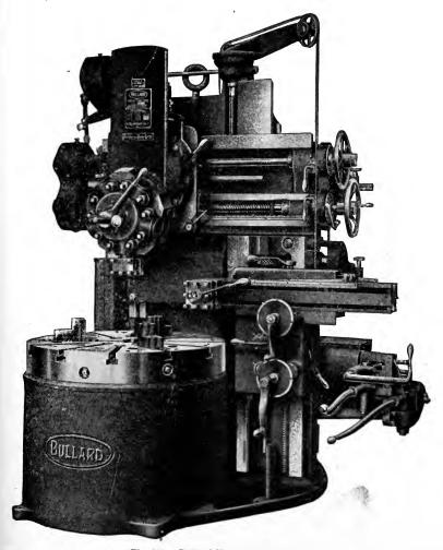
Fig. 353. Bullard Vertical Turret Lathe Courtesy of Bullard Machine Tool Company, Bridgeport, Connecticut
