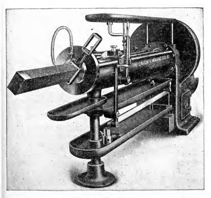
Fig. 365. Typical Broaching Machine Courtesy of LaPointe Machine Tool Company, Hudson, Massachusetts
