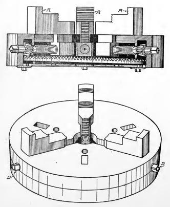
Fig. 103. Combination Chuck
